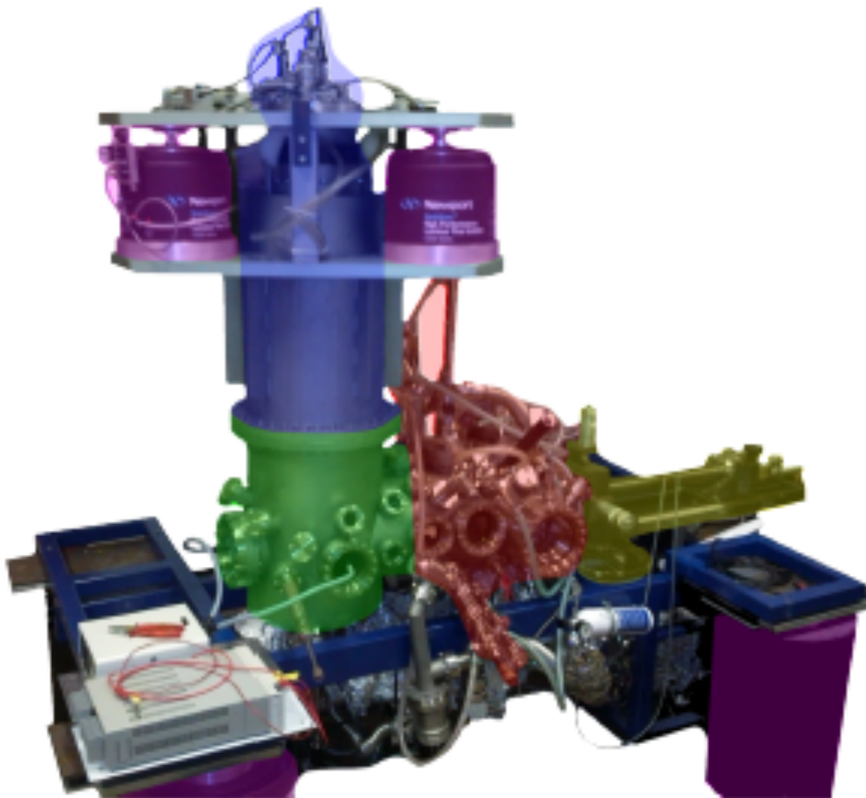
FIGURE 2.3. Image of the LT-STM setup. Parts of the UHV system are depicted: cryostat (blue), STM chamber (green), preparation chamber (red), sample manipulator (yellow), vibration isolation system (magenta).
