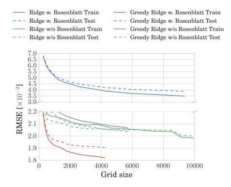
Figure 3.9.: Performance comparison between Ridge and Greedy Ridge regression methods. The Greedy Ridge method clearly shows the ability to create smaller sparse grids with the same representation power.
