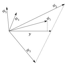
Figure 3.2.: Failure of the forward greedy selection algorithm. The target vector  $\mathbf{y}$  can be represented using the feature vectors  $\boldsymbol{\phi}_2$  and  $\boldsymbol{\phi}_3$ . Nevertheless, the superfluous vector  $\boldsymbol{\phi}_1$  is closer to  $\mathbf{y}$  and is selected first, followed by  $\boldsymbol{\phi}_2$  and  $\boldsymbol{\phi}_3$ . Adapted from T. Zhang (2011).
