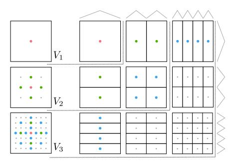
Figure 2.3.: Construction of full grid spaces from hierarchical subspaces. The scheme illustrates the construction of full grid function spaces for maximum levels 1, 2 and 3 (all points) as well as sparse grid function spaces (bold coloured points only).
