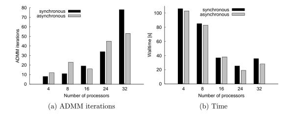
Figure 5.13.: Comparison of the number of ADMM iterations and elapsed time for the synchronous and asynchronous distributed settings. Asynchronous version is superior for more than 24 processors. Source: (Khakhutskyy et al., 2014).
