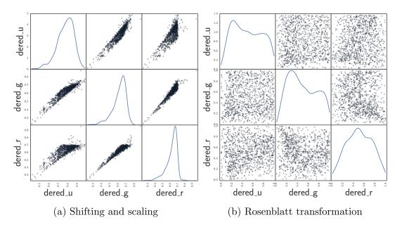
Figure 3.8.: Illustration of the normalisation methods for the first three attributes of the SDSS Data Release 5 dataset. The Rosenblatt transformation removes the correlation between attributes and produces almost uniformly distributed input values.
