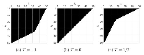
Figure 4.5.: Subspace tableau for a generalised sparse grid with different values of T from (4.29). For T = 0 we obtain the standard regular sparse grid; T > 0 leads to exclusion of hierarchical subspaces from the sparse grid (starting with isotropic ones); T < 0 leads to inclusion of new hierarchical subspaces with the special case  $T = -\infty$ , where it becomes a full grid. Adapted from (Griebel & Knapek, 2000).
