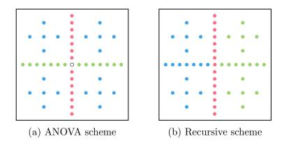
Figure 5.9.: Comparison of the recursive and additive splitting schemes for a sparse grid. Grid points of the same colours are assigned to the same processor. In recursive scheme the processors get either 15 or 17 grid points, in additive scheme either 14 or 20. The imbalance in the ANOVA scheme is higher and grows with the level.
