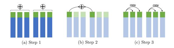
Figure 5.4.: Three-steps communication model for Lines 10 and 20 of Alg. 14 with data partitioning. In the first step, we calculate the sum of large vectors among the processors that share the same data partition (a). In the second step, only the scalar product results are aggregated between the root processes of individual partitions (b). In the last step, the updated values are broadcasted from the roots to all processes in the partitions (c). Source: (Khakhutskyy & Hegland, 2014b).
