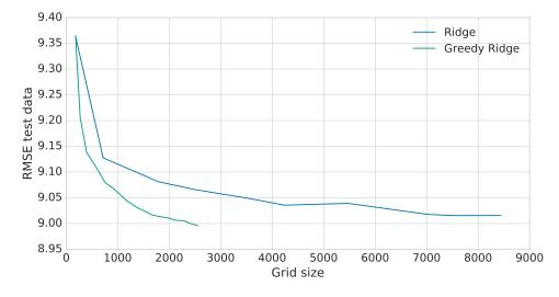
Figure 3.10.: Test error versus sparse grid size for the year prediction challenge MSD. Despite the high dimensionality of the problem large sparse grid models are unnecessary. Greedy Ridge achieves better prediction error with a quarter of the grid size.
