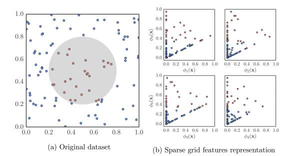
Figure 2.7.: Sparse grid basis function evaluation as feature transformation. Left: red and blue points belong to different classes and cannot be separated by a hyperplane. Right: the same points transformed into a 5-dimensional feature space of a level 2 sparse grid, the problem is separable.
