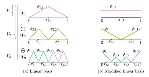
Figure 2.1.: Illustration of one-dimensional hierarchical basis functions up to level 3. All basis functions at the level l span a hierarchical subspace  $W_l$ . The hierarchical subspaces combined together construct the function space  $V_l$ . One-dimensional function spaces for full and sparse grids are indistinguishable.
