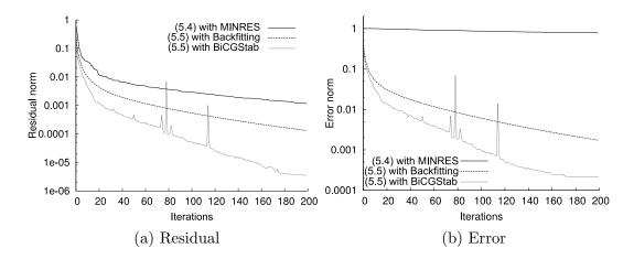
Figure 5.1.: Comparison of problem formulations (5.4) and (5.5) for minimisation of residual and error of a synthetic 100-dimensional dataset from model. Fitting of 1 000 data points was performed using regression cubic splines with  $\lambda = 10^{-7}$  and dof=10. The problem formulation (5.5) is superior to (5.4). MINRES succeeds at minimising the residual this does not affect the prediction error. Source: (Khakhutskyy & Hegland, 2014a).
