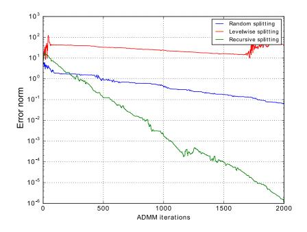
Figure 5.12.: The declining error norm  $\|\mathbf{w}^k - \mathbf{w}^*\|_2$  for Alg. 16 in partially asynchronous setting. The results lie between the synchronous setting in Fig. 5.10a and totally asynchronous setting in Fig. 5.11a. Adopted from (Strauß, 2016).
