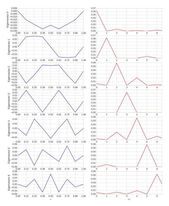
Figure 2.15.: Eigenvectors of a one-dimensional sparse grid smoother. Onedimensional eigenvectors correspond to the different sinus frequencies.
