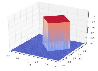
Figure 3.6.: Two-dimensional function with rhombus decision boundaries. This problem poses a challenge for sparse grids since the boundaries are not axis-aligned.
