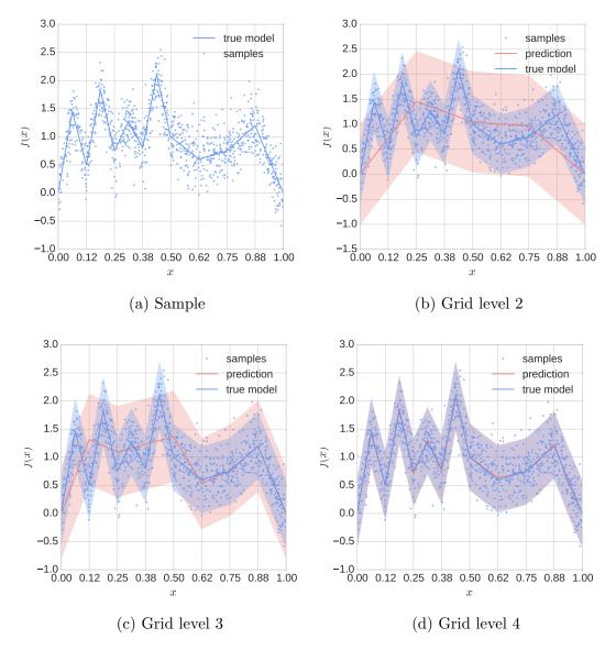
Figure 2.8.: Sparse grid as a Bayesian linear regressor with depicted uncertainty. Figures show the true and predicted functions as well as the 95% confidence intervals of the posterior and data distributions. Lower grid level corresponds to higher overall variance. Level 4 of the esimtated model matches the level of the true model, in this case the agreement between the distributions becomes almost perfect.
