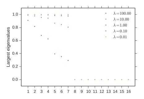
Figure 2.14.: Eigenvalues for one-dimensional sparse grid with different regularisation parameters  $\lambda$ . As regularisation matrix we used identity matrix. The nonzero eigenvalues are very close to 1 even for relatively high  $\lambda$  of 0.1 and 0.01.
