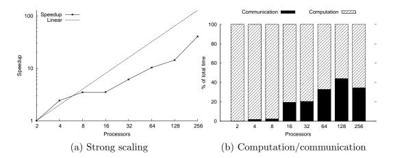
Figure 5.6.: Scaling properties of Alg. 14. On the left: strong scaling results for the Million Songs dataset with 88 features and 463715 examples. On the right: the computation-to-communication relationship for different number of processors. Due to the limited size of the dataset we show the strong scaling results of up to 256 processors. Source: (Khakhutskyy & Hegland, 2014b).
