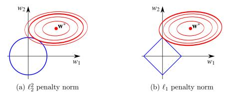
Figure 3.3.: Parameter estimation for lasso and ridge regression. The ball of the penalisation term  $\mathcal{B}$  is depicted in blue and the level-set of L is depicted in red. At the optimal point the level-set is tangential to  $\mathcal{B}$ .
