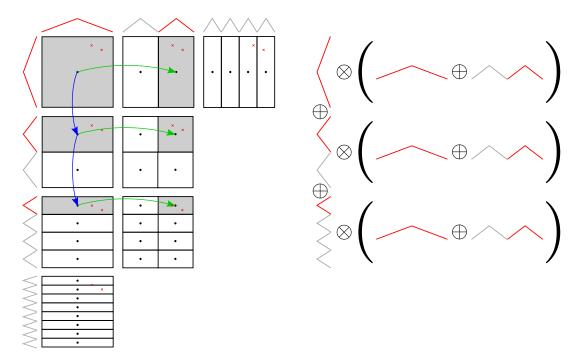
Figure 2.12.: Illustration of the recursive fast kernel evaluation scheme using distributive law. The algorithm starts with iteration through the dimension 0 and then continues the recursive descent into other dimensions for all function levels that still cover both points.
