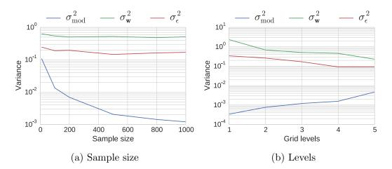
Figure 2.9.: Dependence of variance components from level and sample size. Left: for the fixed grid level as the sample size grows the model variance  $\sigma_{\rm mod}^2$  vanishes and the additive data noise  $\sigma_{\varepsilon}^2$  dominates the variance of the predictive distribution. Right: for the fixed dataset size as the grid level increases the optimal hyperparameters decrease while the model variance increases.
