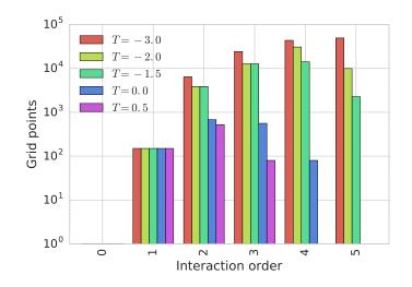
Figure 4.6.: Number of grid points in different interaction orders for generalised sparse grids. For a regular sparse grid with T = 0 most of the points concentrate in the 2-order and 3-order interactions. For T > 0 the number of points in higher interaction terms diminishes. For T < 0 the number of points in higher interactions explodes. The shape of the point distribution remains the same.
