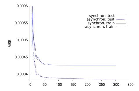
Figure 5.14.: Convergence of ADMM algorithm based on grid splitting for the synchronous and asynchronous settings. The results are indistinguishable. Adopted from (Khakhutskyy et al., 2014).
