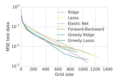
Figure 3.7.: Test error for different refinement methods. The greedy lasso method outperforms other methods once the grid becomes larger than 400 grid points. For more than 1000 grid points elastic-net shows superior results.
