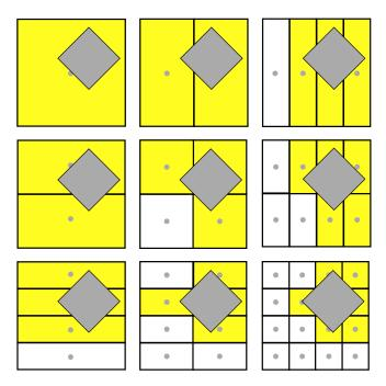
Figure 3.1.: Adaptive sparse grid for decision boundary identification. In order to adapt the model to the manifold, we need to identify only those basis functions which intersect the decision boundaries in every hierarchical subspace.
