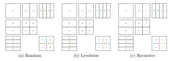
Figure 5.8.: Sparse grid splitting schemes. Different colours identify the sparse grid functions assigned to the same processor.
