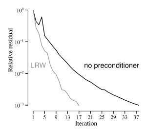
Figure 5.2.: Comparison of the relative residual for BiCGStab without preconditioner and with the LRW preconditioner. LRW facilitates the convergence significantly. Source: (Uphoff, 2015, Fig. 8.1.).
