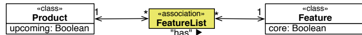
Figure 4.48.: A Product has no variability in it, it has a final list of Features.
