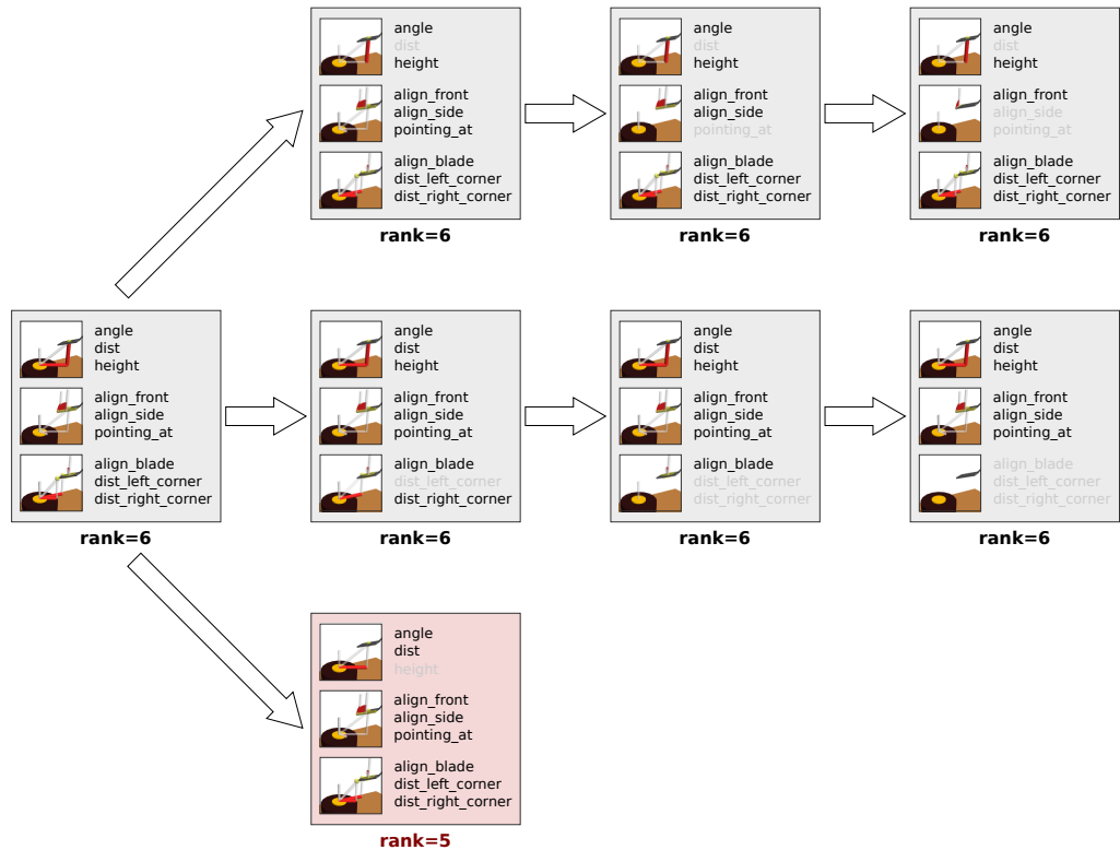
Figure 4.14.: Sample constraint elimination processes: Top row: The distance, pointing_at- and align_side task functions are removed. Part of the spatula orientation is described by the distance of the spatula corners to the center. Middle row: The extra task functions distance_left_corner, distance_right_corner and align_blade are removed. This yields the VKC-like task function as described previously. Bottom row: The height task function cannot be removed without lowering the rank. This task function is non-redundant.
