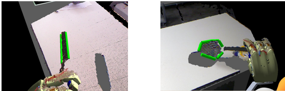
Figure 2.4.: Geometric line features that were detected in a long spatula and a skimmer.
