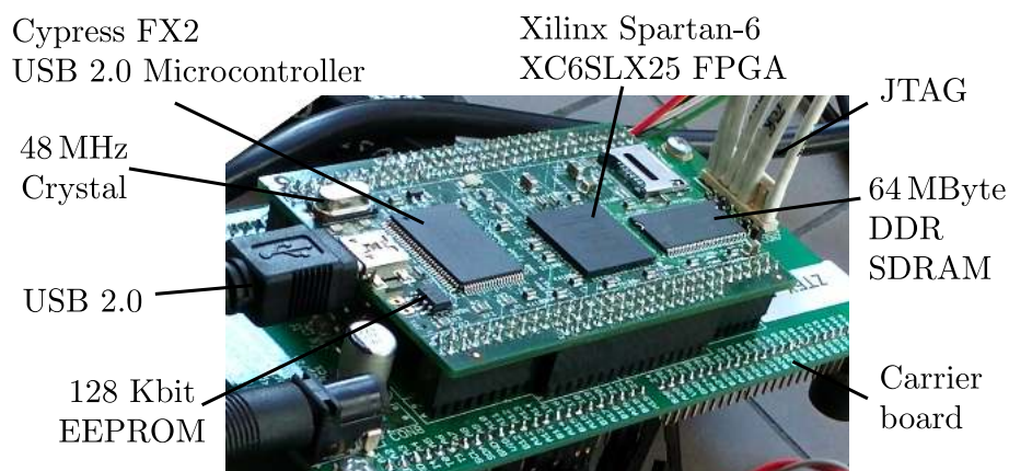
Figure 3.12: ZTEX USB-FPGA-Module 1.11c with Xilinx Spartan-6 LX25.
