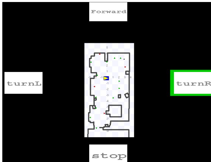
Figure 5.12: Simulated environment with SSVEP stimuli overlaid at the sides of the display. The stimuli constellation allows for intuitive interaction.
