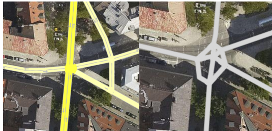
Figure 2-6: Differences in modelling of road networks between two map vendors
