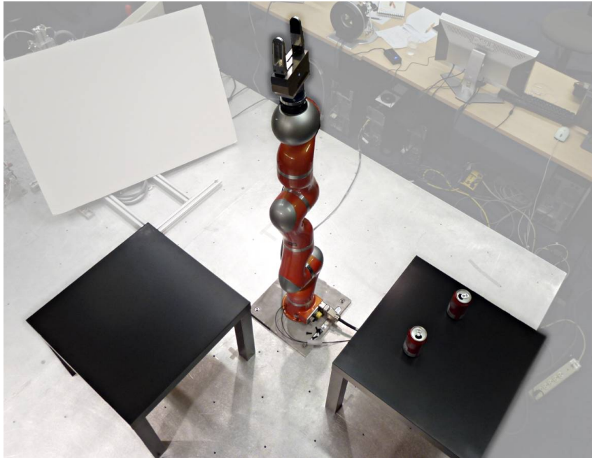
Figure 3.1: Implementation of a FORCE SENSING instance with two objects, a torque-sensing compliant manipulator and a force-controlled parallel gripper [7, 9]. The LBR4 robot is supposed to transfer beverage containers to another table, and it must hold containers upright to prevent spilling unless they are known to be empty.
