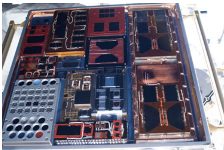
Fig. 5-10: MISSE-8 experiment with three ChipSats on the left side of the panel on the bottom-middle, taken from Manchester (2015, p.21)
