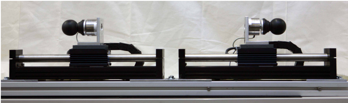
Figure 4.2: One-DoF linear axis teleoperation system.
