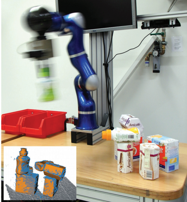
Fig. 14. The setup of the vision-based grasping experiments. The robot has grasped a green soda club bottle and is about to put it in the further red bin. The Kinect sensor can be seen in the upper right corner. In the lower left corner, the range image and the recognized models are shown (before the bottle has been taken away) from a viewpoint close to that of the sensor.
