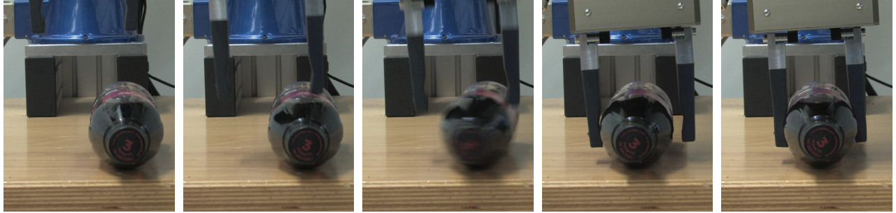
Fig. 7. Grasping behavior with low stiffness. Note that despite the imprecise object pose the robot is able to grasp the bottle.
