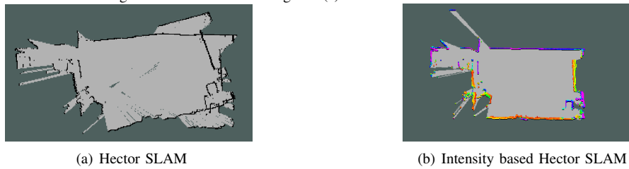
Fig. 6. A specific scenario highlighting the advantage of intensity based Hector SLAM over standard Hector SLAM. The field of view (FOV) of the scanner based on the minimum and maximum angle is [-1.047 \ 1.047] radians. The dimensions of the room are approximately 8.5m \times 5.5m . a) Hector SLAM failed to create a consistent map as it could not find sufficient geometric features for pose estimation while turning at two different corners. b) Intensity based Hector SLAM succeeded in generating a consistent map as it additionally utilizes surface reflectivities for pose estimation.
