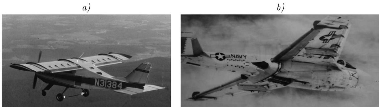
**Figure 2.11:** WVU Flight Demonstrator (a) and Grumman A-6A (b) as examples for flying circulation control demonstrators (LOTH, 2006)
