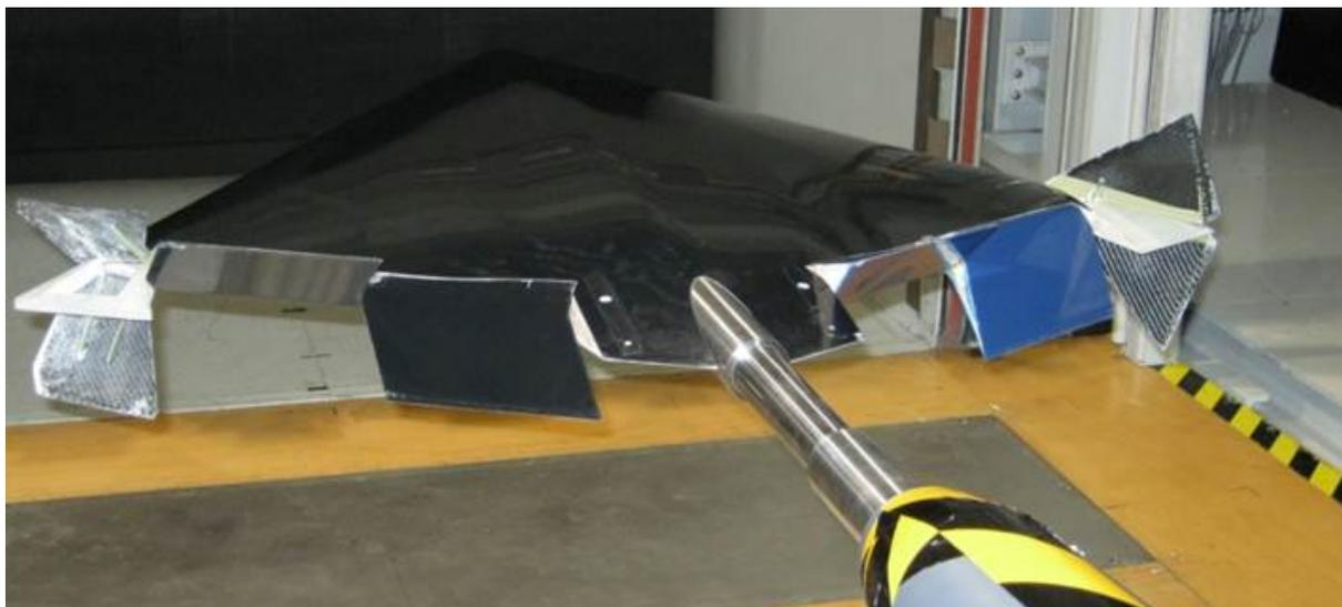
**Figure 4.4:** SAGITTA wind tunnel model with conventional plain flaps and two different types of tip split flaps (left: abandoned concept, right: investigated vortex flap concept)
