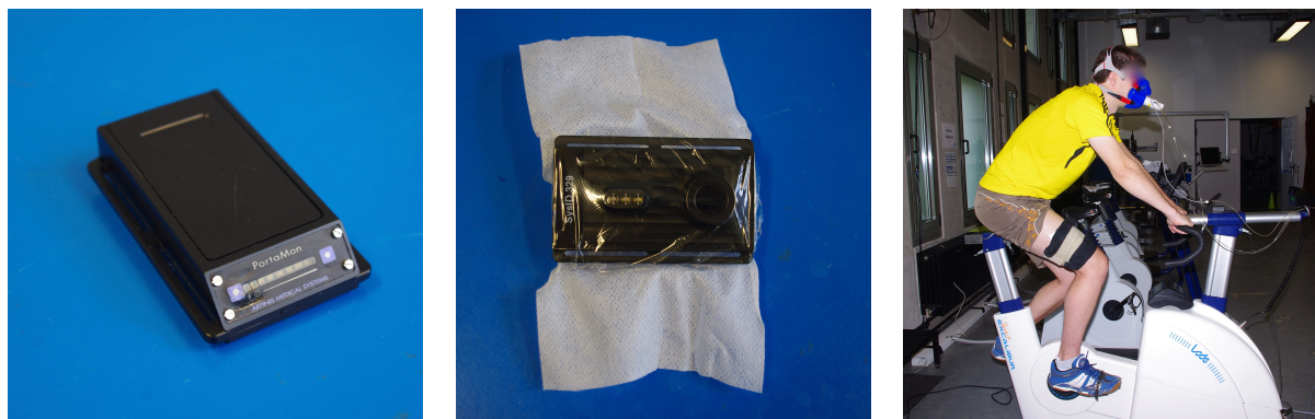
Figure 5 Left panel: NIRS device „portamon“, Artinis (Zetten, NL); middle panel: NIRS device upside down (three transmitter optodes and one receiver optode), covered in plastic foil for protection against humidity and placed on adhesive tape; right panel: subject sitting on a bicycle ergometer (Lode excalibur, Groningen, NL), wearing the NIRS device (covered to avoid influences of ambient light) on the right thigh and a spirometry mask.
