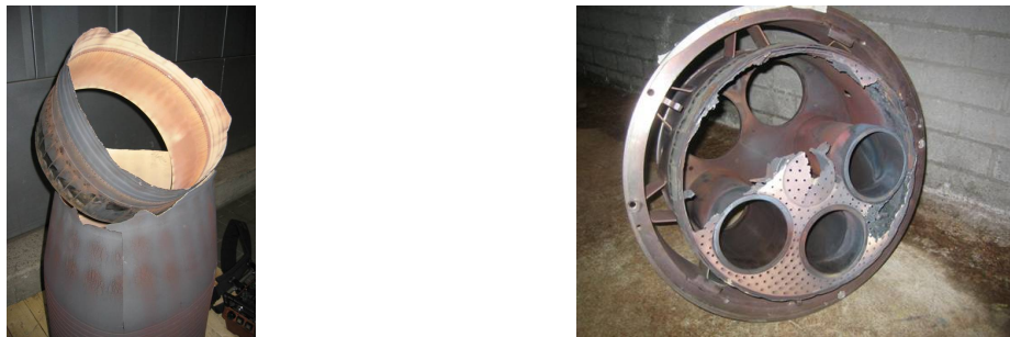
Figure 1.1: Damages of a gas turbine liner (left) and combustor face plate (right) due to thermoacoustic instability. 1
