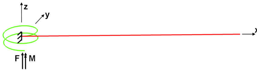
Figure 3.20: Problem setup: Initially straight beam bent by a discrete end-moment and -force.
