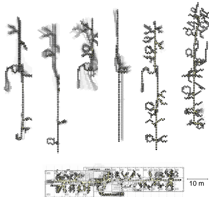
Figure 6.9: Six FootSLAM maps of DLR building 103 (on the top) and their combined map. The building layout has been manually aligned to the FootSLAM map and is shown only as a reference.
