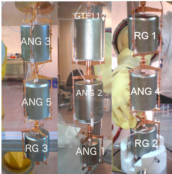
(a) Three detector strings with eight detectors from enriched Germanium and one from natural material
