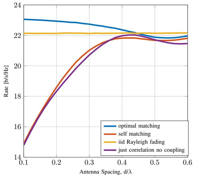
Fig. 4: Rates with receiver CSI vs. antenna spacing
