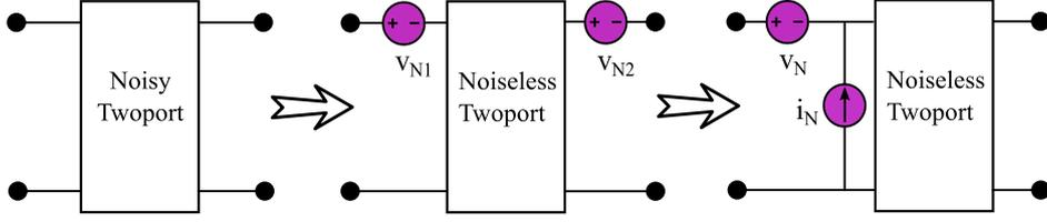
Fig. 1: Noisy fourpole models and equivalent circuits
