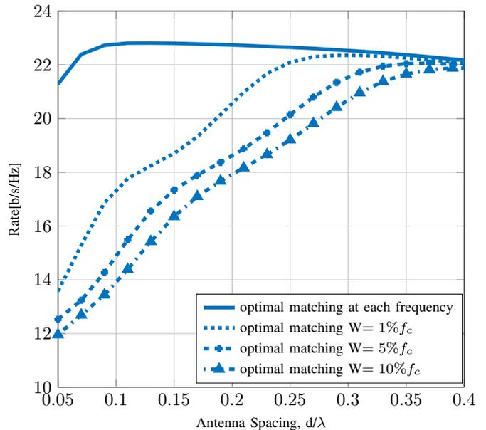
Fig. 7: Rates vs. antenna spacing with varying relative bandwidth
