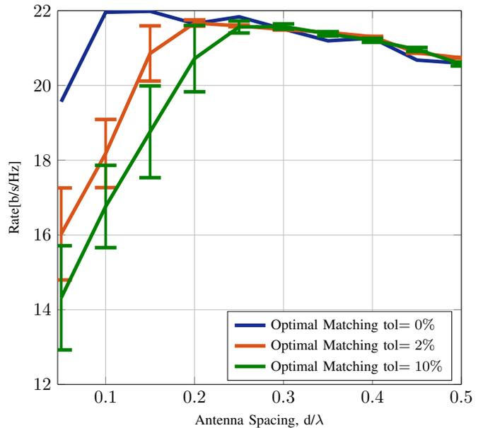
Fig. 6: Rates vs. antenna spacing with element tolerances
