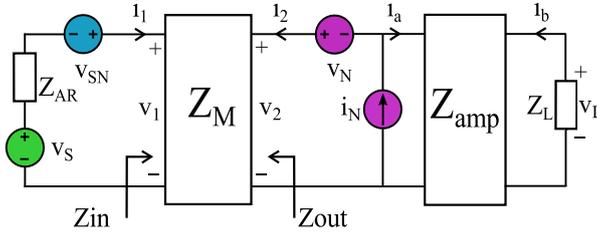
Fig. 2: Single antenna front-end receiver with impedance matching
