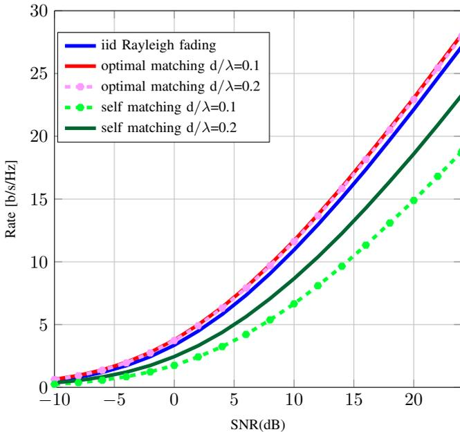
Fig. 5: Rates with receiver CSI vs. SNR
