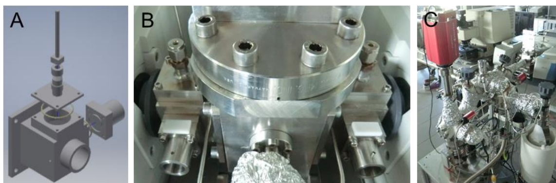
Figure 6-8: (A) Schematic collocation of all essential components of an optical device for holding a Ge-mirror, which reflects UV-Vis-light into a vacuum infrared cell made of stainless steel for in situ investigations of self-supported wafers. (B) Photograph of the infrared cell and the Ge-mirror holders and (C) of the whole infrared spectroscopy setup.
