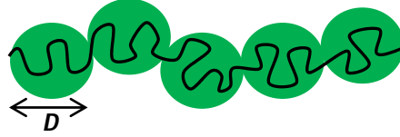
Fig. 2.2: Schematic representation of the polyelectrolyte chain as an array of electrostatic blobs of size D .
