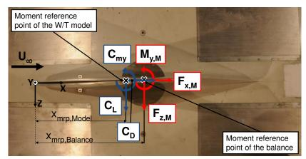
Figure 3.14: Determination of the aerodynamic coefficients at the AVT-183 W/T model.
