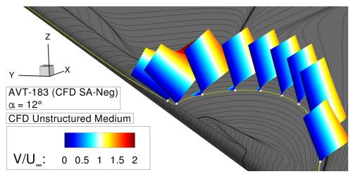
(b) Skin-friction lines including near-wall velocity profiles colored by absolute velocity  $V/U_{\infty}$  that are located along one particular skin-friction line (front view).
