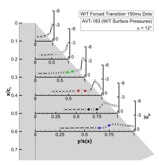
Figure 5.10: Flow physics analysis of the AVT-183 configuration – Surface pressure coefficient  $\overline{c_p}$  versus semi-span y/s(x) at  $\alpha = 12^{\circ}$ .
