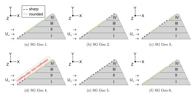
Figure 1.10: Spanwise-varying leading-edge contours of the SAGITTA configuration (right wing).
