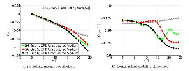
Figure 6.20: Longitudinal aerodynamic coefficients of configurations SG Geo 5 and SG Geo 6 – Pitching-moment coefficient  $C_{my}$  and derivative  $C_{my,\alpha}$  versus angle of attack  $\alpha$ .
