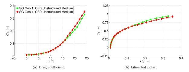
Figure 6.39: Longitudinal aerodynamic coefficients of configuration SG Geo 4 – Drag coefficient  $C_D$  versus angle of attack  $\alpha$  and Lilienthal polar  $C_L$  versus  $C_D$ .
