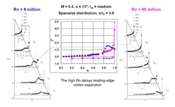
Figure 2.5: Reynolds number effect on blunt leading-edge vortex separation [89].
