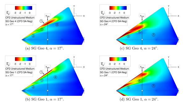
Figure 6.42: Longitudinal stability investigation of configuration SG Geo 4 – Surface pressure coefficient  $\overline{c_p}$ .
