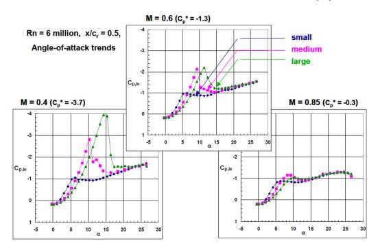
Figure 2.9: Bluntness and Mach number effect on leading-edge vortex separation [87].
