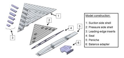
Figure 3.3: AVT-183 W/T model components.
