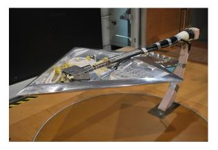
Figure 3.8: SAGITTA W/T model without the pressure side shell.
