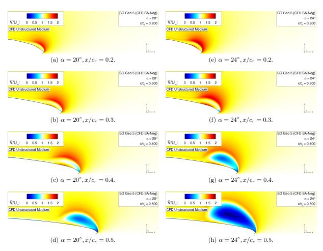
Figure 6.15: Flow physics analysis of configuration SG Geo 5 – Absolute velocity contours  $\overline{V}/U_{\infty}$ .
