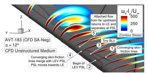
(a) Skin-friction lines including axial vorticity contours  $\omega_x \cdot l_\mu/U_\infty$ . The contour levels have been adjusted for the following analysis.
