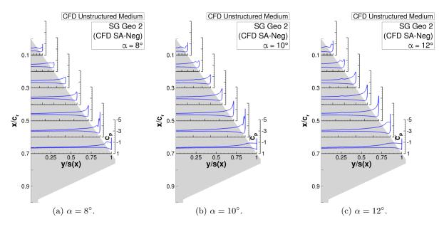
Figure 6.23: Flow physics analysis of configuration SG Geo 2 – Surface pressure coefficient  $\overline{c_p}$  versus semi-span y/s(x).
