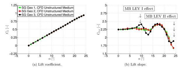
Figure 6.30: Longitudinal aerodynamic coefficients of configurations SG Geo 2 and SG Geo 3 – Lift coefficient  $C_L$  and derivative  $C_{L,\alpha}$  versus angle of attack  $\alpha$ .
