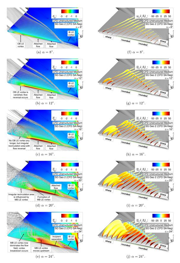
Figure 6.24: Flow physics analysis of configuration SG Geo 2 – Surface pressure coefficient  $\overline{c_p}$  including field streamlines, and axial vorticity contours  $\overline{\omega_x} \cdot l_{\mu}/U_{\infty}$ .
