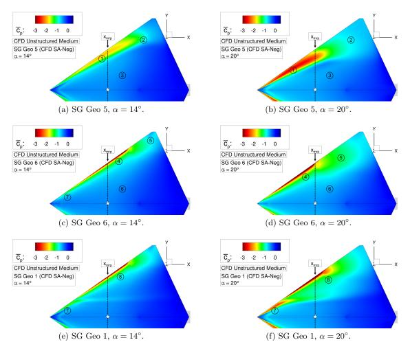
Figure 6.22: Longitudinal stability investigation of configurations SG Geo 5 and SG Geo 6 – Surface pressure coefficient  $\overline{c_p}$ .
