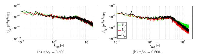
Figure 5.16: Flow physics analysis of the AVT-183 configuration – Power spectral densities of velocity fluctuations at  $\alpha = 12^{\circ}$  outside of the leading-edge vortex. The locations can be observed from Figure 5.14e and Figure 5.14f.
