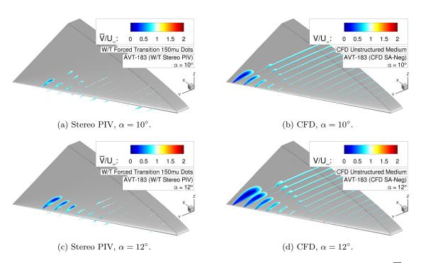
Figure 5.24: CFD validation of the AVT-183 configuration – Absolute velocity contours  $\overline{V}/U_{\infty}$ .
