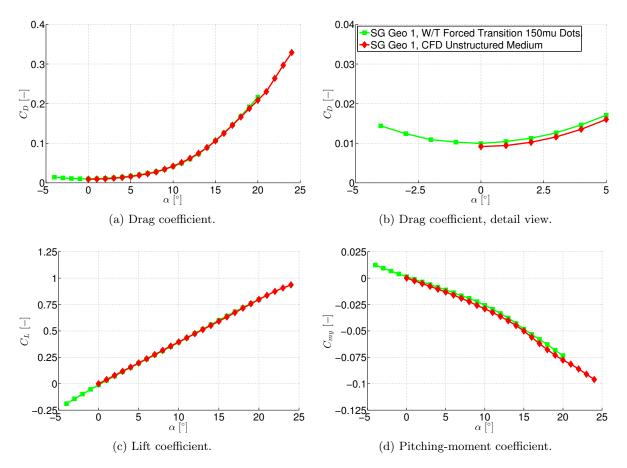
Figure 6.3: CFD validation of configuration SG Geo 1 – Longitudinal aerodynamic coefficients versus angle of attack  $\alpha$ .
