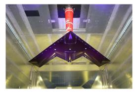
Figure 1.4: SACCON UCAV low-speed wind tunnel model [23].
