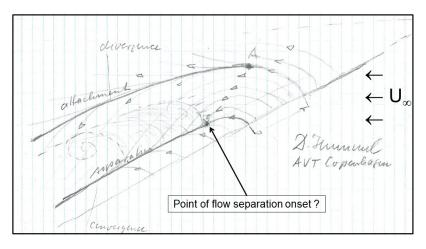
Figure 1.7: Scenario of the flow separation onset at a non-slender wing with rounded leading edge [63].
