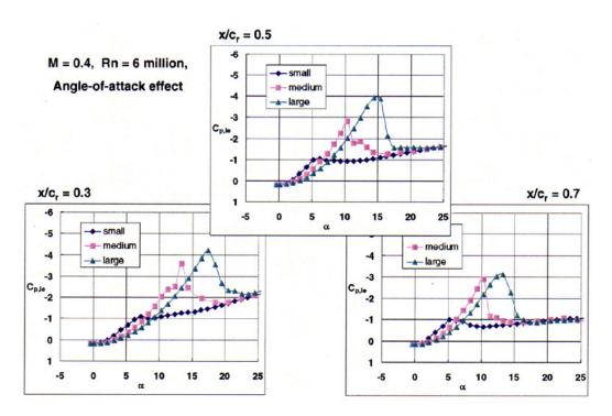
Figure 2.8: Bluntness effect on leading-edge vortex separation [88].
