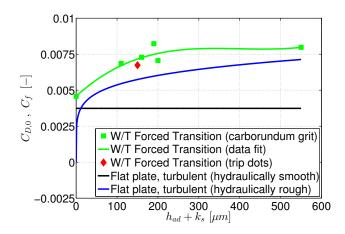
Figure 5.3: Leading-edge roughness effects at the AVT-183 configuration — Zero-lift drag coefficient  $C_{D,0}$  and skin-friction coefficient  $C_f$  versus total roughness height  $h_{ad} + k_s$ .
