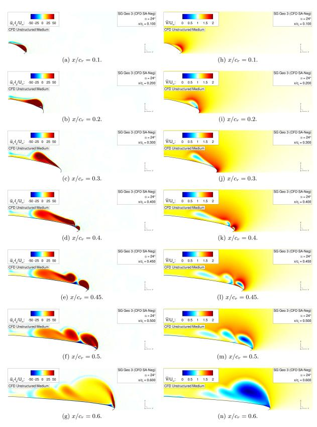
Figure 6.29: Flow physics analysis of configuration SG Geo 3 – Axial vorticity contours  $\overline{\omega_x} \cdot l_{\mu}/U_{\infty}$ and absolute velocity contours  $\overline{V}/U_{\infty}$  at  $\alpha = 24^{\circ}$ .
