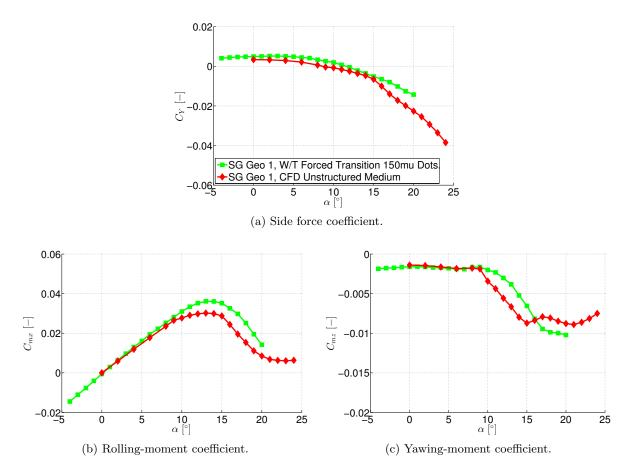
Figure C.1: CFD validation – Lateral aerodynamic coefficients versus angle of attack  $\alpha$  at  $\beta = -10^{\circ}$ , configuration SG Geo 1.
