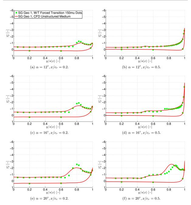
Figure C.2: CFD validation – Surface pressure coefficient  $\overline{c_p}$  versus semi-span y/s(x) at  $\beta = -10^{\circ}$ , configuration SG Geo 1.
