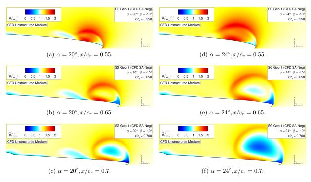
Figure 6.13: Flow physics analysis of configuration SG Geo 1 – Absolute velocity contours  $\overline{V}/U_{\infty}$  at  $\beta = -10^{\circ}$ .
