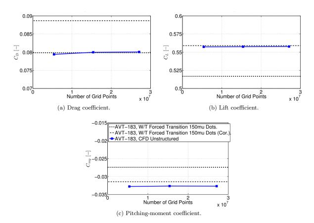
Figure 5.21: CFD validation of the AVT-183 configuration – Longitudinal aerodynamic coefficients for different grid resolutions at  $\alpha = 12^{\circ}$ .
