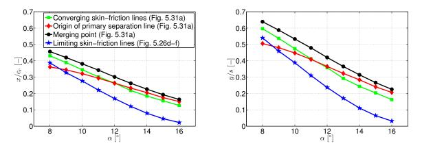
Figure 5.36: Flow separation onset characteristics of the AVT-183 configuration – Location of characteristic points versus angle of attack  $\alpha$ .
