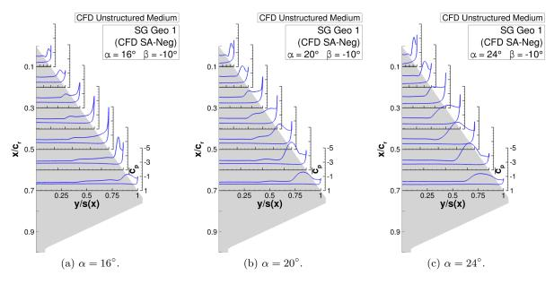
Figure 6.12: Flow physics analysis of configuration SG Geo 1 – Surface pressure coefficient  $\overline{c_p}$  versus semi-span y/s(x) at  $\beta = -10^{\circ}$ .
