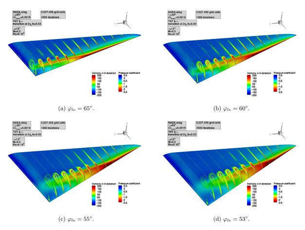
Figure 2.12: Wing planform and relative thickness effect on leading-edge vortex separation [9].
