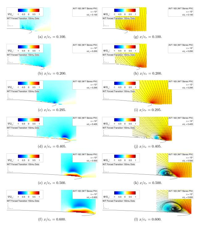
Figure 5.12: Flow physics analysis of the AVT-183 configuration – Lateral velocity component contours  $\overline{v}/U_{\infty}$  and normal velocity component contours  $\overline{w}/U_{\infty}$  at  $\alpha = 12^{\circ}$ .
