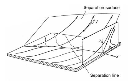
Figure 2.2: Nature of three-dimensional flow separation [18].
