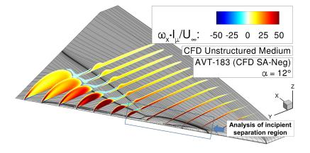
Figure 5.30: Flow separation onset characteristics of the AVT-183 configuration – Axial vorticity contours  $\omega_x \cdot l_{\mu}/U_{\infty}$  including skin-friction lines at  $\alpha = 12^{\circ}$ .
