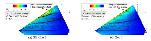
Figure 6.27: Flow physics analysis of configuration SG Geo 3 – Surface pressure coefficient  $\overline{c_p}$  including skin-friction lines at  $\alpha = 12^{\circ}$ .
