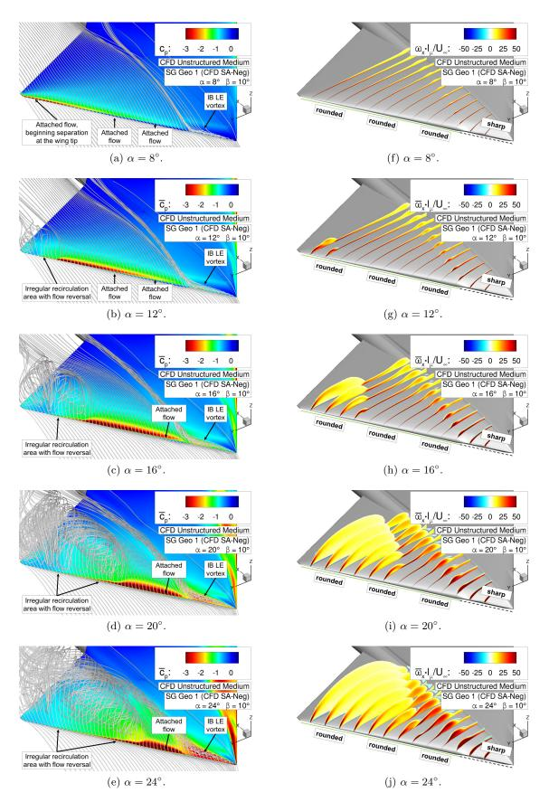
Figure C.3: Flow physics analysis of configuration SG Geo 1 – Surface pressure coefficient  $\overline{c_p}$  including streamlines, and axial vorticity contours  $\omega_x \cdot l_\mu/U_\infty$  at  $\beta = 10^\circ$ .
