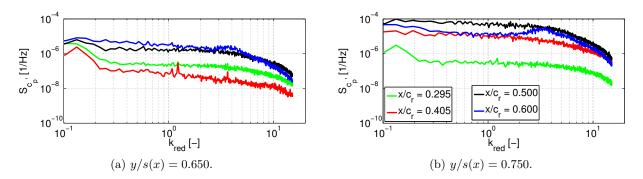
Figure 5.13: Flow physics analysis of the AVT-183 configuration – Power spectral densities of unsteady surface pressure fluctuations at  $\alpha = 12^{\circ}$ .
