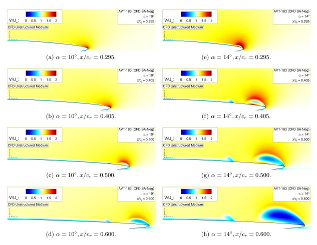
Figure 5.28: Flow physics analysis of the AVT-183 configuration – Absolute velocity contours  $V/U_{\infty}$ .
