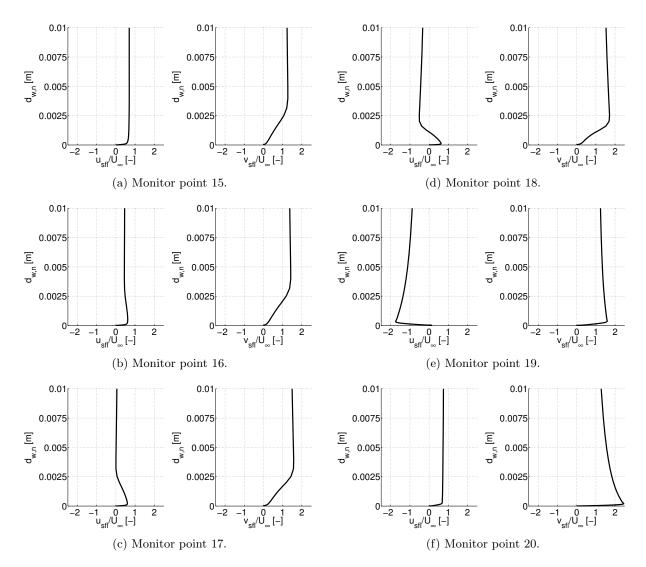
Figure 5.35: Flow separation onset characteristics of the AVT-183 configuration at  $\alpha = 12^{\circ}$  – Near-wall velocity profiles in streamwise and crossflow direction along one particular skin-friction line.
