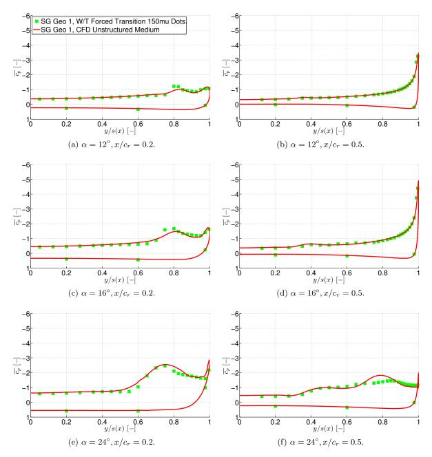
Figure 6.7: CFD validation of configuration SG Geo 1 – Surface pressure coefficient  $\overline{c_p}$  versus semi-span y/s(x).
