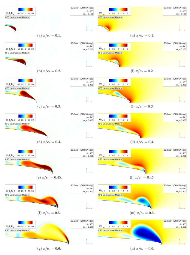
Figure 6.10: Flow physics analysis of configuration SG Geo 1 – Axial vorticity contours  $\overline{\omega_x} \cdot l_\mu / U_\infty$ and absolute velocity contours  $\overline{V}/U_\infty$  at  $\alpha = 24^\circ$ .
