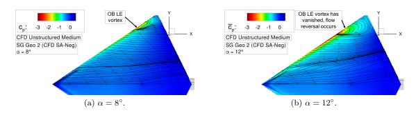
Figure 6.25: Flow physics analysis of configuration SG Geo 2 – Surface pressure coefficient  $\overline{c_p}$  including skin-friction lines.
