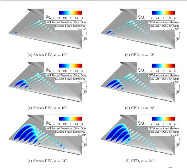
Figure 6.6: CFD validation of configuration SG Geo 1 – Absolute velocity contours  $\overline{V}/U_{\infty}$ .
