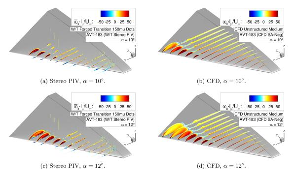
Figure 5.23: CFD validation of the AVT-183 configuration – Axial vorticity contours  $\overline{\omega_x} \cdot l_{\mu}/U_{\infty}$ .
