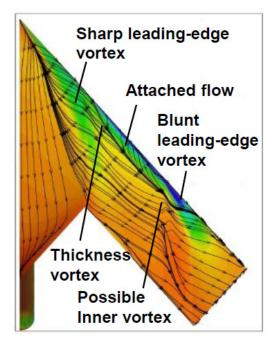
Figure 1.5: SACCON vortex flow phenomena,  $\alpha = 16.83^{\circ}$  [39, 86].
