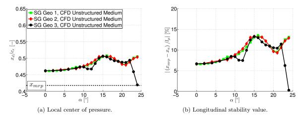
Figure 6.33: Longitudinal stability investigation of configurations SG Geo 2 and SG Geo 3 – Local center of pressure  $x_d/c_r$  and stability value  $|(x_{mrp} - x_n)/l_{\mu}|$  vs. angle of attack  $\alpha$ .
