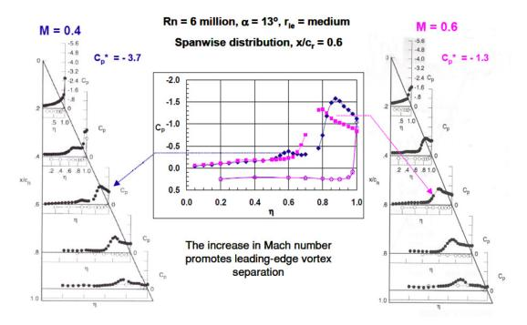
Figure 2.7: Mach number effect on blunt leading-edge vortex separation [89].
