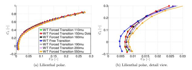
Figure 5.2: Leading-edge roughness effects at the AVT-183 configuration — Lilienthal polar  $C_L$  versus  $C_D$ .
