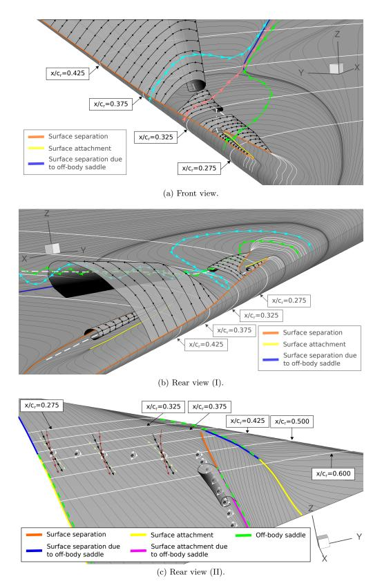
Figure 5.38: Flow topology interpretation of the AVT-183 configuration at  $\alpha=12^\circ$  – Three-dimensional views.
