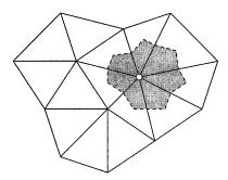
Figure 4.4: Dual grid approach – Secondary grid data based on the cell-vertex grid metric [44].
