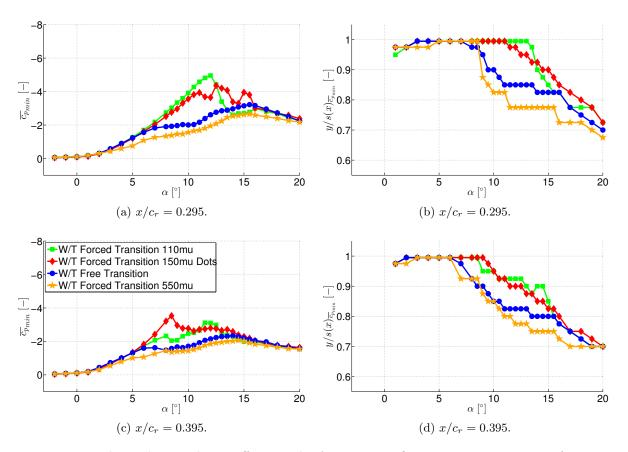
Figure 5.5: Leading-edge roughness effects at the AVT-183 configuration – Minimum surface pressure coefficient  $\overline{c_{p,min}}$  and corresponding spanwise locations versus angle of attack  $\alpha$ .
