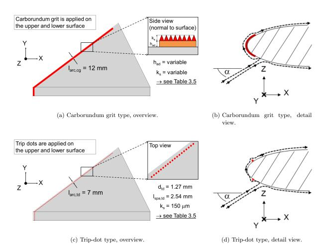
Figure 3.12: Geometric properties of the applied trip strips at the AVT-183 W/T model.
