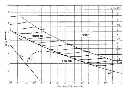
Figure 3.10: Skin-friction coefficient versus Reynolds number on a flat plate at zero incidence and zero pressure gradient, see Truckenbrodt [131].
