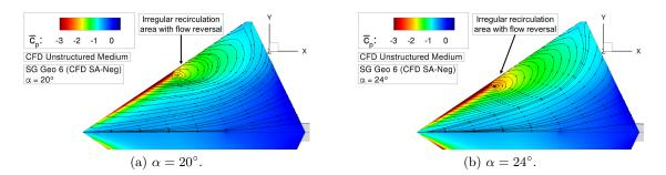
Figure 6.17: Flow physics analysis of configuration SG Geo 6 – Surface pressure coefficient  $\overline{c_p}$  including skin-friction lines.
