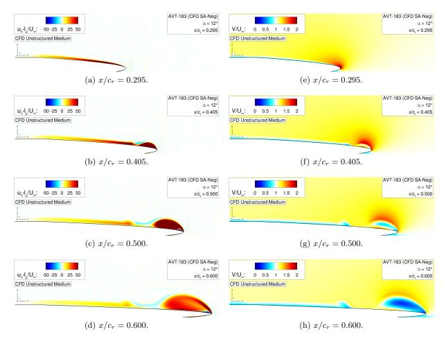
Figure 5.29: Flow physics analysis of the AVT-183 configuration – Axial vorticity contours  $\omega_x \cdot l_{\mu}/U_{\infty}$  and absolute velocity contours  $V/U_{\infty}$  at  $\alpha = 12^{\circ}$ .
