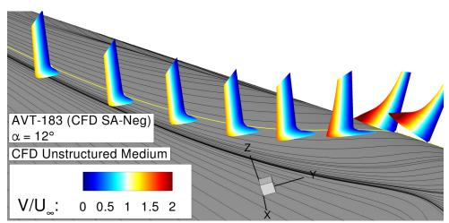
(c) Skin-friction lines including near-wall velocity profiles colored by absolute velocity  $V/U_{\infty}$  that are located along one particular skin-friction line (rear view).
