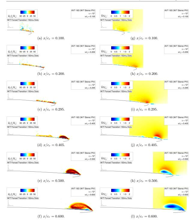
Figure 5.11: Flow physics analysis of the AVT-183 configuration – Axial vorticity contours  $\overline{\omega_x} \cdot l_{\mu}/U_{\infty}$  and absolute velocity contours  $\overline{V}/U_{\infty}$  at  $\alpha = 12^{\circ}$ .
