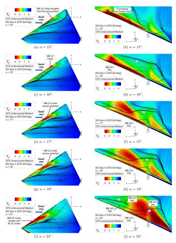
Figure 6.36: Flow physics analysis of configuration SG Geo 4 – Surface pressure coefficient  $\overline{c_p}$  including skin-friction lines.
