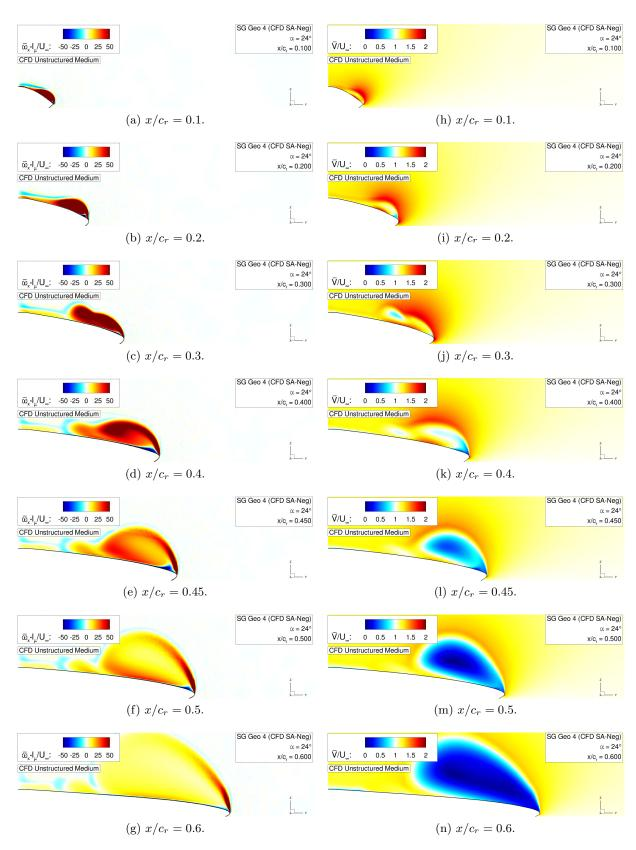
Figure 6.37: Flow physics analysis of configuration SG Geo 4 – Axial vorticity contours  $\overline{\omega_x} \cdot l_{\mu}/U_{\infty}$ and absolute velocity contours  $\overline{V}/U_{\infty}$  at  $\alpha = 24^{\circ}$ .
