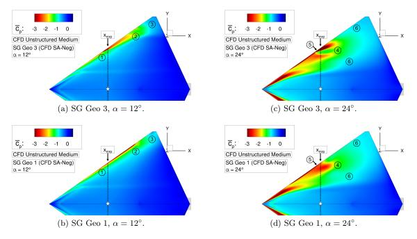
Figure 6.34: Longitudinal stability investigation of configuration SG Geo 3 – Surface pressure coefficient  $\overline{c_p}$ .
