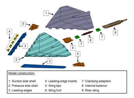
Figure 3.7: SAGITTA W/T model components.
