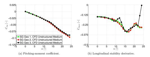
Figure 6.32: Longitudinal aerodynamic coefficients of configurations SG Geo 2 and SG Geo 3 – Pitching-moment coefficient  $C_{my}$  and derivative  $C_{my,\alpha}$  versus angle of attack  $\alpha$ .
