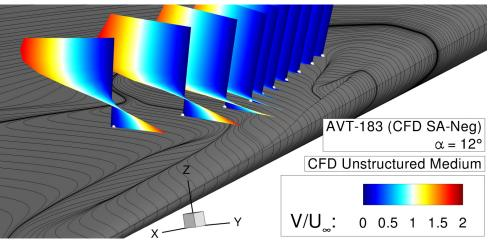
(c) Skin-friction lines including near-wall velocity profiles colored by absolute velocity  $V/U_{\infty}$  that are located along the leading-edge vortex core (rear view).
