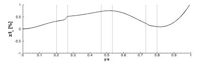
Figure 1.11: Leading-edge twist modification (nose coordinate) for configuration SG Geo 4.
