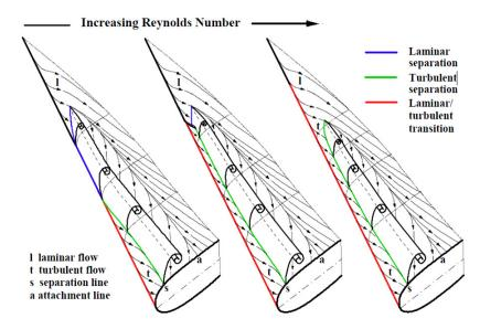
Figure 2.6: Reynolds number effect on vortex formation along rounded leading edges [57].
