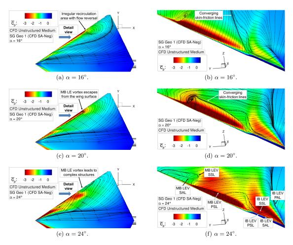
Figure 6.9: Flow physics analysis of configuration SG Geo 1 – Surface pressure coefficient  $\overline{c_p}$  including skin-friction lines.
