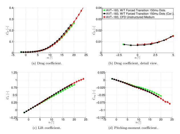
Figure 5.22: CFD validation of the AVT-183 configuration – Longitudinal aerodynamic coefficients versus angle of attack  $\alpha$ .
