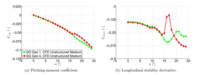
Figure 6.40: Longitudinal aerodynamic coefficients of configuration SG Geo 4 – Pitching-moment coefficient  $C_{my}$  and derivative  $C_{my,\alpha}$  versus angle of attack  $\alpha$ .
