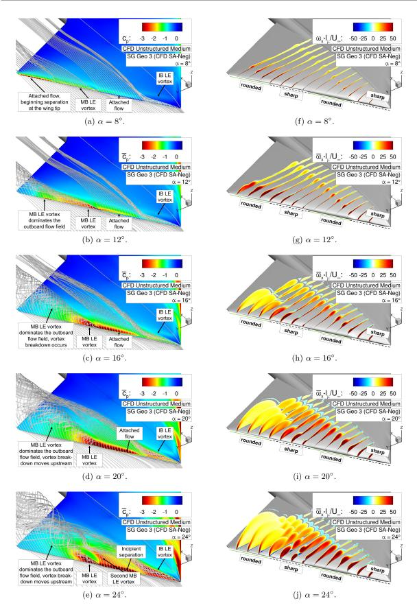
Figure 6.26: Flow physics analysis of configuration SG Geo 3 – Surface pressure coefficient  $\overline{c_p}$  including field streamlines, and axial vorticity contours  $\overline{\omega_x} \cdot l_{\mu}/U_{\infty}$ .
