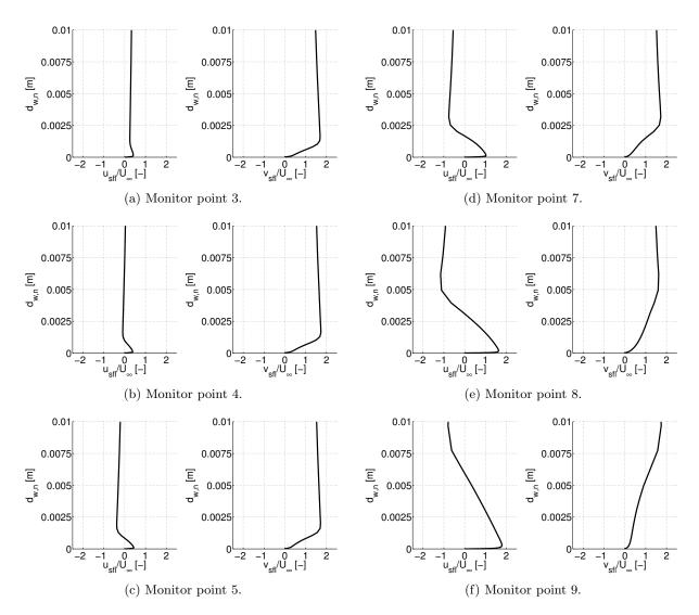
Figure 5.33: Flow separation onset characteristics of the AVT-183 configuration at  $\alpha = 12^{\circ}$  – Near-wall velocity profiles in streamwise and crossflow direction along the leadingedge vortex core.
