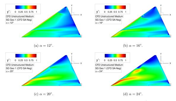
Figure 6.1: CFD validation of configuration SG Geo 1 – Computed  $y^+$  levels.
