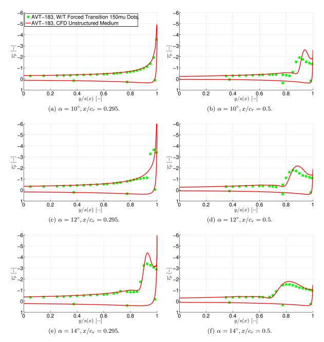
Figure 5.25: CFD validation of the AVT-183 configuration – Surface pressure coefficient  $\overline{c_p}$  versus semi-span y/s(x).
