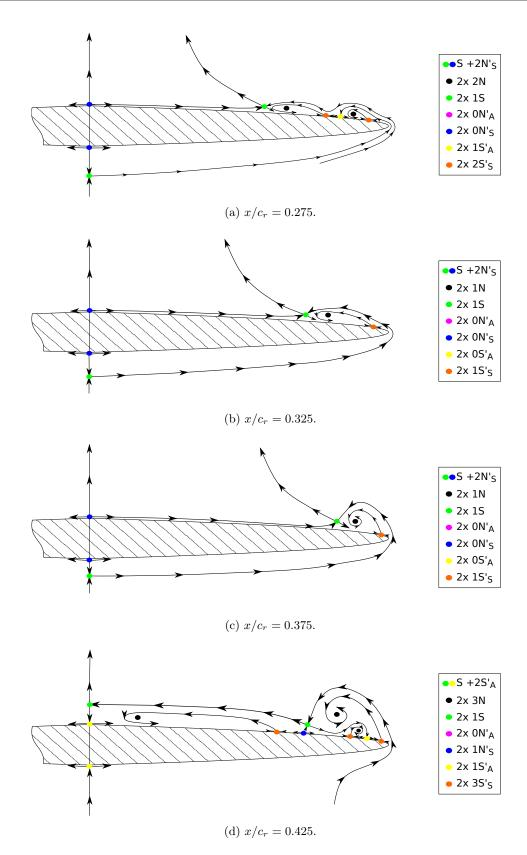
Figure 5.39: Flow topology interpretation of the AVT-183 configuration at  $\alpha = 12^{\circ}$  – Sectional cuts (I).
