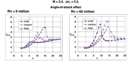
Figure 2.10: Bluntness and Reynolds number effect on leading-edge vortex separation [88].
