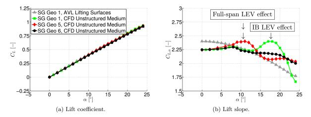
Figure 6.18: Longitudinal aerodynamic coefficients of configurations SG Geo 5 and SG Geo 6 – Lift coefficient  $C_L$  and derivative  $C_{L,\alpha}$  versus angle of attack  $\alpha$ .
