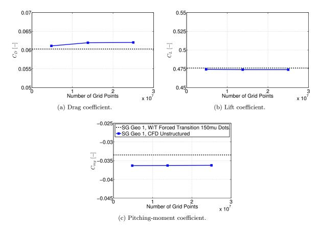
Figure 6.2: CFD validation of configuration SG Geo 1 – Longitudinal aerodynamic coefficients for different grid resolutions at  $\alpha = 12^{\circ}$ .
