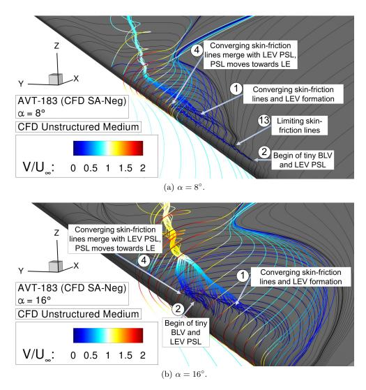
Figure 5.37: Flow separation onset characteristics of the AVT-183 configuration – Skin-friction lines including field streamlines colored by absolute velocity  $V/U_{\infty}$ .
