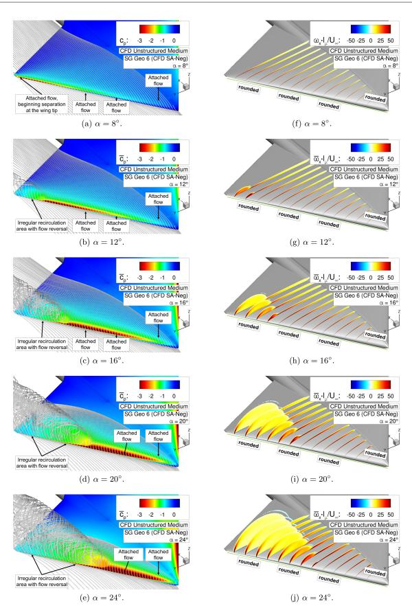
Figure 6.16: Flow physics analysis of configuration SG Geo 6 – Surface pressure coefficient  $\overline{c_p}$  including field streamlines, and axial vorticity contours  $\overline{\omega_x} \cdot l_{\mu}/U_{\infty}$ .
