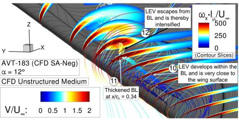
(c) Skin-friction lines including axial vorticity contours  $\omega_x \cdot l_\mu/U_\infty$  and field streamlines colored by absolute velocity  $V/U_\infty$ .
