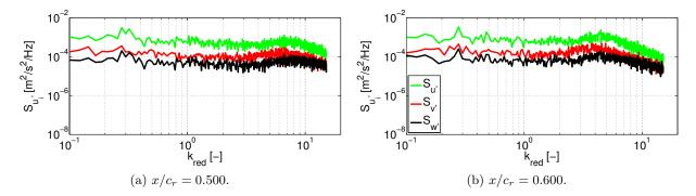
Figure 5.15: Flow physics analysis of the AVT-183 configuration – Power spectral densities of velocity fluctuations at  $\alpha = 12^{\circ}$  close to local turbulence maxima. The locations can be observed from Figure 5.14e and Figure 5.14f.
