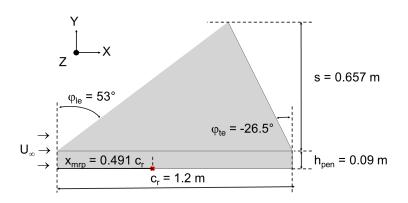
Figure 3.2: AVT-183 W/T model, top view xy plane.
