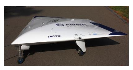
Figure 1.8: SAGITTA demonstrator configuration.
