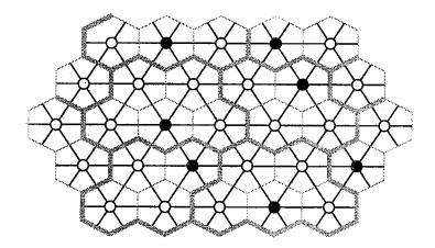
Figure 4.5: Multigrid method – Agglomeration of control volumes to form a coarser mesh [44].
