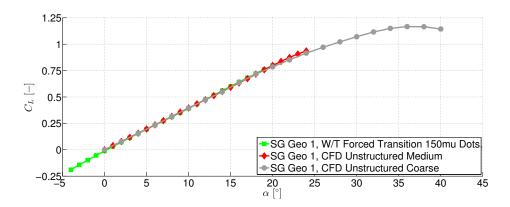
Figure 6.4: CFD validation of configuration SG Geo 1 – Lift coefficient versus angle of attack  $\alpha$ .
