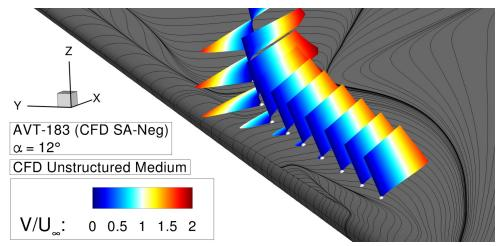
(b) Skin-friction lines including near-wall velocity profiles colored by absolute velocity  $V/U_{\infty}$  that are located along the leading-edge vortex core (front view).
