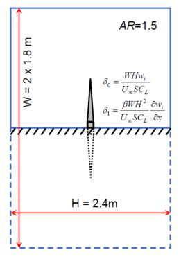
Figure B.1: Sketch of mirrored W/T test section for the applied W/T correction [35].
