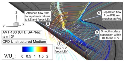
(b) Skin-friction lines including field streamlines colored by absolute velocity  $V/U_{\infty}$ . The field streamlines have been released with  $d_{w,n} = 0.005 \ mm$ .
