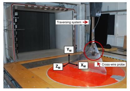
Figure 3.18: Overview of the applied hot-wire set-up within the W/T facility A of TUM-AER.
