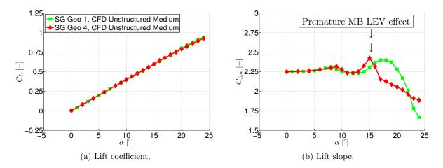
Figure 6.38: Longitudinal aerodynamic coefficients of configuration SG Geo 4 – Lift coefficient  $C_L$  and derivative  $C_{L,\alpha}$  versus angle of attack  $\alpha$ .
