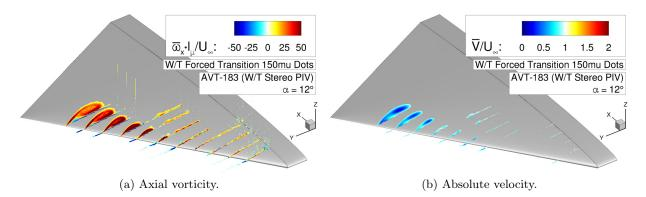
Figure 5.9: Flow physics analysis of the AVT-183 configuration – Axial vorticity contours  $\overline{\omega_x} \cdot l_{\mu}/U_{\infty}$  and absolute velocity contours  $\overline{V}/U_{\infty}$  at  $\alpha = 12^{\circ}$ .
