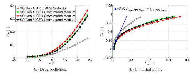
Figure 6.19: Longitudinal aerodynamic coefficients of configurations SG Geo 5 and SG Geo 6 – Drag coefficient  $C_D$  versus angle of attack  $\alpha$  and Lilienthal polar  $C_L$  versus  $C_D$ .
