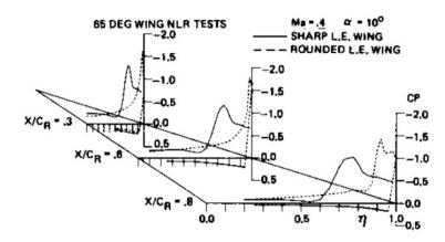
Figure 1.2: Effect of the leading-edge shape on the pressure distribution at the VFE-1 configuration for Ma = 0.4,  $Re_{mac} = 9 \cdot 10^6$  and  $\alpha = 10^\circ$  [36].
