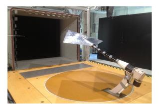
Figure 3.9: SAGITTA W/T model within the W/T facility A of TUM-AER.
