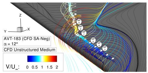
(a) Skin-friction lines including field streamlines colored by absolute velocity  $V/U_{\infty}$  and monitor points for near-wall velocity profile evaluation.
