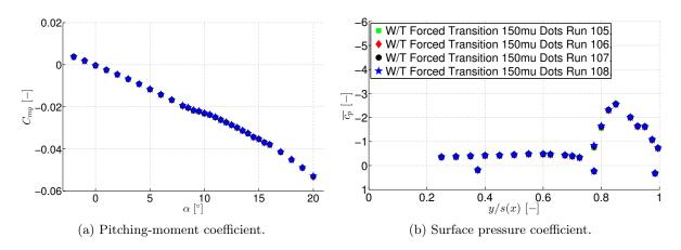
Figure 5.7: Short-term repeatability issues of case W/T Forced Transition 150mu Dots — Pitching-moment coefficient  $C_{my}$  versus angle of attack  $\alpha$  and surface pressure coefficient  $\overline{c_p}$  versus semi-span y/s(x) at  $\alpha = 14^{\circ}$  and  $x/c_r = 0.405$ .
