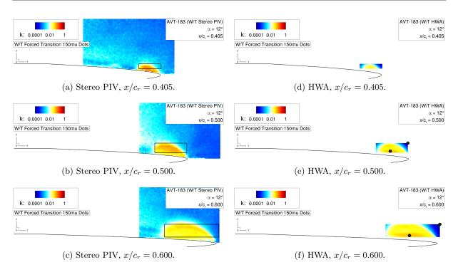
Figure 5.14: Flow physics analysis of the AVT-183 configuration – Turbulent kinetic energy contours k at  $\alpha = 12^{\circ}$ .
