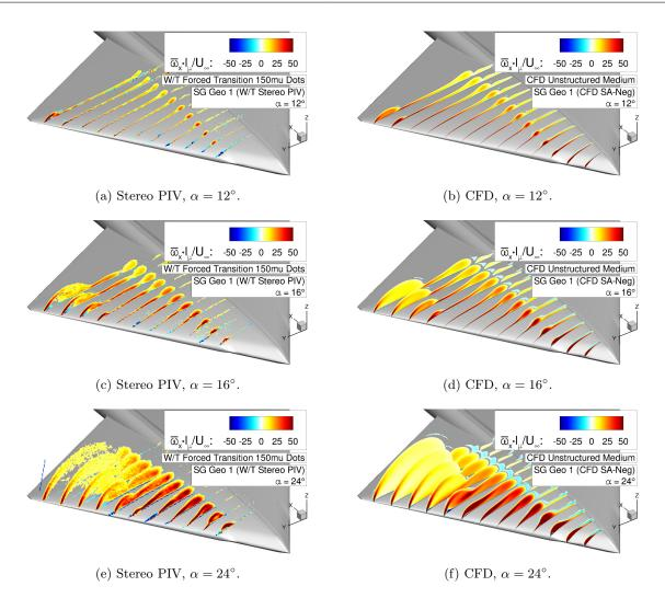
Figure 6.5: CFD validation of configuration SG Geo 1 – Axial vorticity contours  $\overline{\omega_x} \cdot l_\mu/U_\infty$ .
