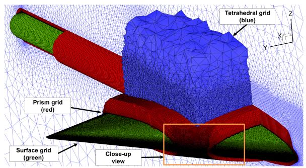
(a) Overall break-up of the different grid types.
