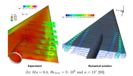
Figure 1.3: Flow field characteristics and flow topology of the VFE-2 configuration with rounded leading edges.
