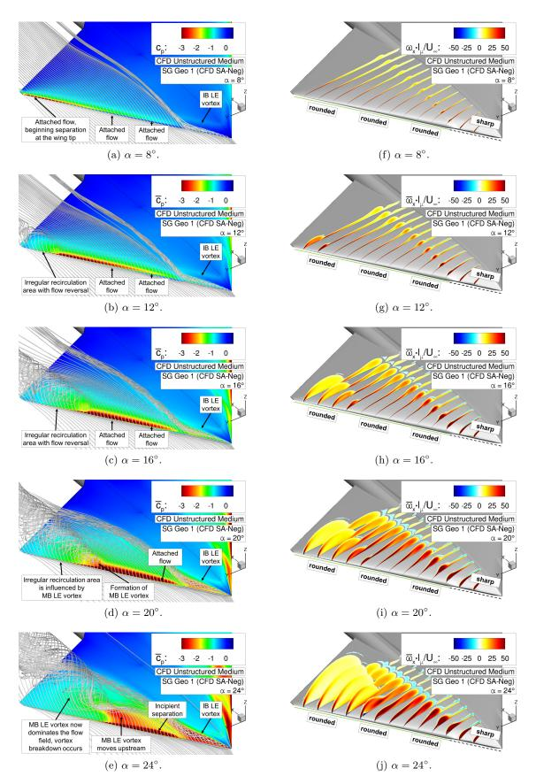
Figure 6.8: Flow physics analysis of configuration SG Geo 1 – Surface pressure coefficient  $\overline{c_p}$  including field streamlines, and axial vorticity contours  $\overline{\omega_x} \cdot l_{\mu}/U_{\infty}$ .
