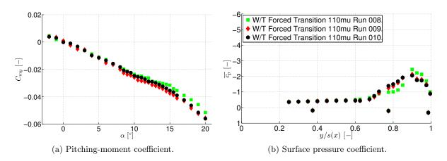
Figure 5.6: Short-term repeatability issues of case W/T Forced Transition 110mu — Pitchingmoment coefficient  $C_{my}$  versus angle of attack  $\alpha$  and surface pressure coefficient  $\overline{c_p}$ versus semi-span y/s(x) at  $\alpha = 14^{\circ}$  and  $x/c_r = 0.405$ .
