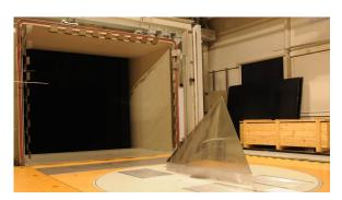
Figure 3.5: AVT-183 W/T model within the W/T facility A of TUM-AER.
