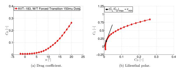
Figure 5.18: Longitudinal aerodynamic characteristics of the AVT-183 configuration — Drag coefficient  $C_D$  versus angle of attack  $\alpha$  and Lilienthal polar  $C_L$  versus  $C_D$ .
