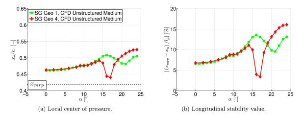
Figure 6.41: Longitudinal stability investigation of configuration SG Geo 4 – Local center of pressure  $x_d/c_r$  and stability value  $|(x_{mrp} - x_n)/l_{\mu}|$  vs. angle of attack  $\alpha$ .
