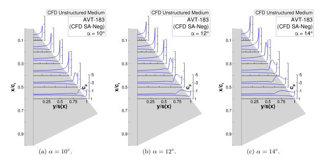
Figure 5.27: Flow physics analysis of the AVT-183 configuration – Surface pressure coefficient  $c_p$  versus semi-span y/s(x).
