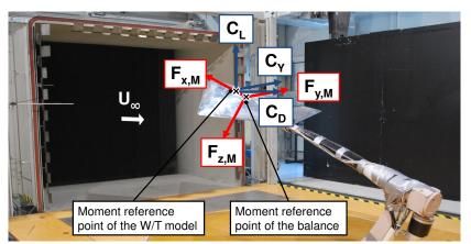
Figure 3.15: Determination of the aerodynamic coefficients at the SAGITTA W/T model.
