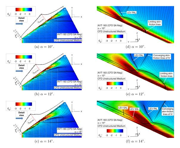
Figure 5.26: Flow physics analysis of the AVT-183 configuration – Surface pressure coefficient  $c_p$  including skin-friction lines.
