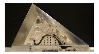
Figure 3.4: AVT-183 W/T model without the pressure side shell.
