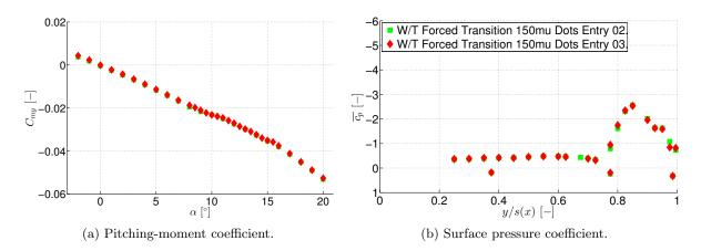
Figure 5.8: Long-term repeatability issues of case W/T Forced Transition 150mu Dots — Pitching-moment coefficient  $C_{my}$  versus angle of attack  $\alpha$  and surface pressure coefficient  $\overline{c_p}$  versus semi-span y/s(x) at  $\alpha = 14^{\circ}$  and  $x/c_r = 0.405$ .
