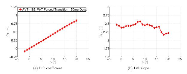
Figure 5.17: Longitudinal aerodynamic characteristics of the AVT-183 configuration — Lift coefficient  $C_L$  and derivative  $C_{L,\alpha}$  versus angle of attack  $\alpha$ .
