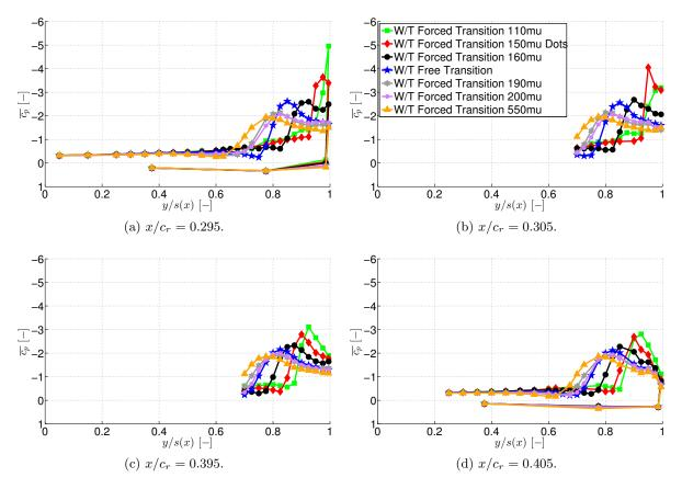
Figure 5.4: Leading-edge roughness effects at the AVT-183 configuration – Surface pressure coefficient  $\overline{c_p}$  versus semi-span y/s(x) at  $\alpha = 12^{\circ}$ .
