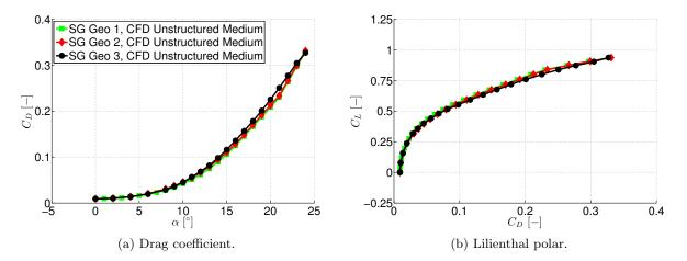
Figure 6.31: Longitudinal aerodynamic coefficients of configurations SG Geo 2 and SG Geo 3 – Drag coefficient  $C_D$  versus angle of attack  $\alpha$  and Lilienthal polar  $C_L$  versus  $C_D$ .
