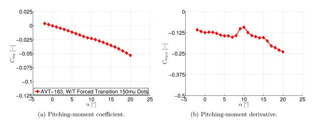
Figure 5.19: Longitudinal aerodynamic characteristics of the AVT-183 configuration – Pitchingmoment coefficient  $C_{my}$  and derivative  $C_{my,\alpha}$  versus angle of attack  $\alpha$ .
