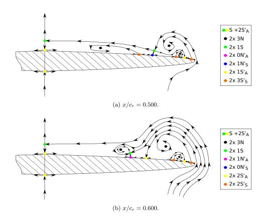
Figure 5.40: Flow topology interpretation of the AVT-183 configuration at  $\alpha = 12^{\circ}$  – Sectional cuts (II).
