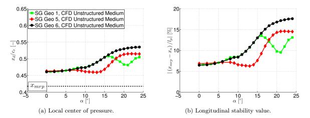
Figure 6.21: Longitudinal stability investigation of configurations SG Geo 5 and SG Geo 6 – Local center of pressure  $x_d/c_r$  and stability value  $|(x_{mrp} - x_n)/l_{\mu}|$  vs. angle of attack  $\alpha$ .
