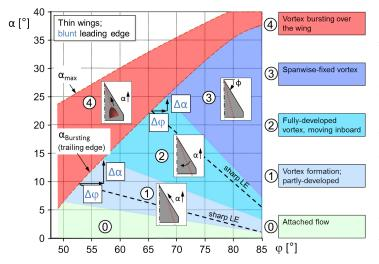
Figure 2.11: Wing planform and angle-of-attack effect on leading-edge vortex separation [19].
