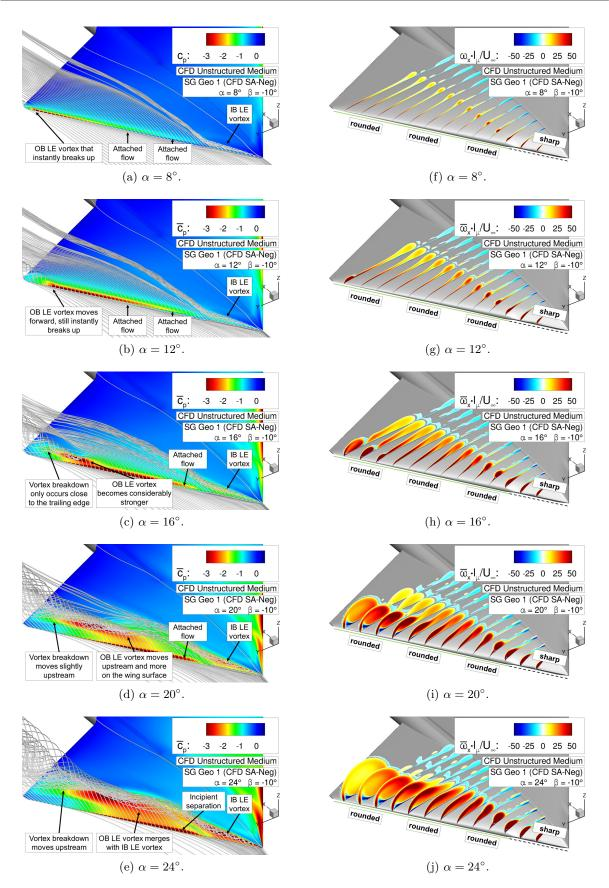
Figure 6.11: Flow physics analysis of configuration SG Geo 1 – Surface pressure coefficient  $\overline{c_p}$  including field streamlines, and axial vorticity contours  $\overline{\omega_x} \cdot l_{\mu}/U_{\infty}$  at  $\beta = -10^{\circ}$ .
