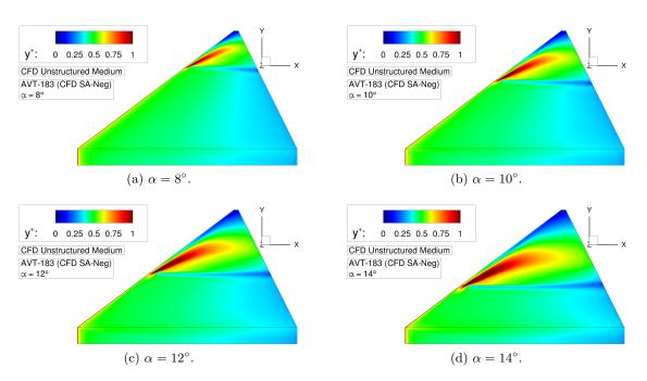
Figure 5.20: CFD validation of the AVT-183 configuration – Computed  $y^+$  levels.
