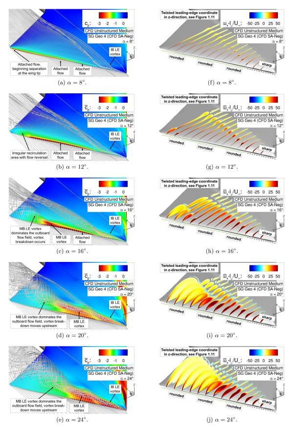
Figure 6.35: Flow physics analysis of configuration SG Geo 4 – Surface pressure coefficient  $\overline{c_p}$  including field streamlines, and axial vorticity contours  $\overline{\omega_x} \cdot l_{\mu}/U_{\infty}$ .
