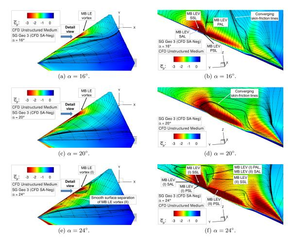
Figure 6.28: Flow physics analysis of configuration SG Geo 3 – Surface pressure coefficient  $\overline{c_p}$  including skin-friction lines.
