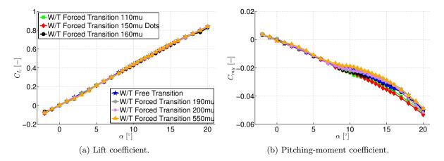
Figure 5.1: Leading-edge roughness effects at the AVT-183 configuration — Lift coefficient  $C_L$ and pitching-moment coefficient  $C_{my}$  versus angle of attack  $\alpha$ .
