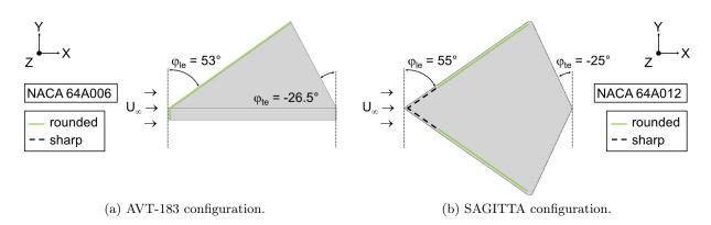
Figure 1.9: Planform comparison of the analyzed diamond wing configurations, top view xy plane.
