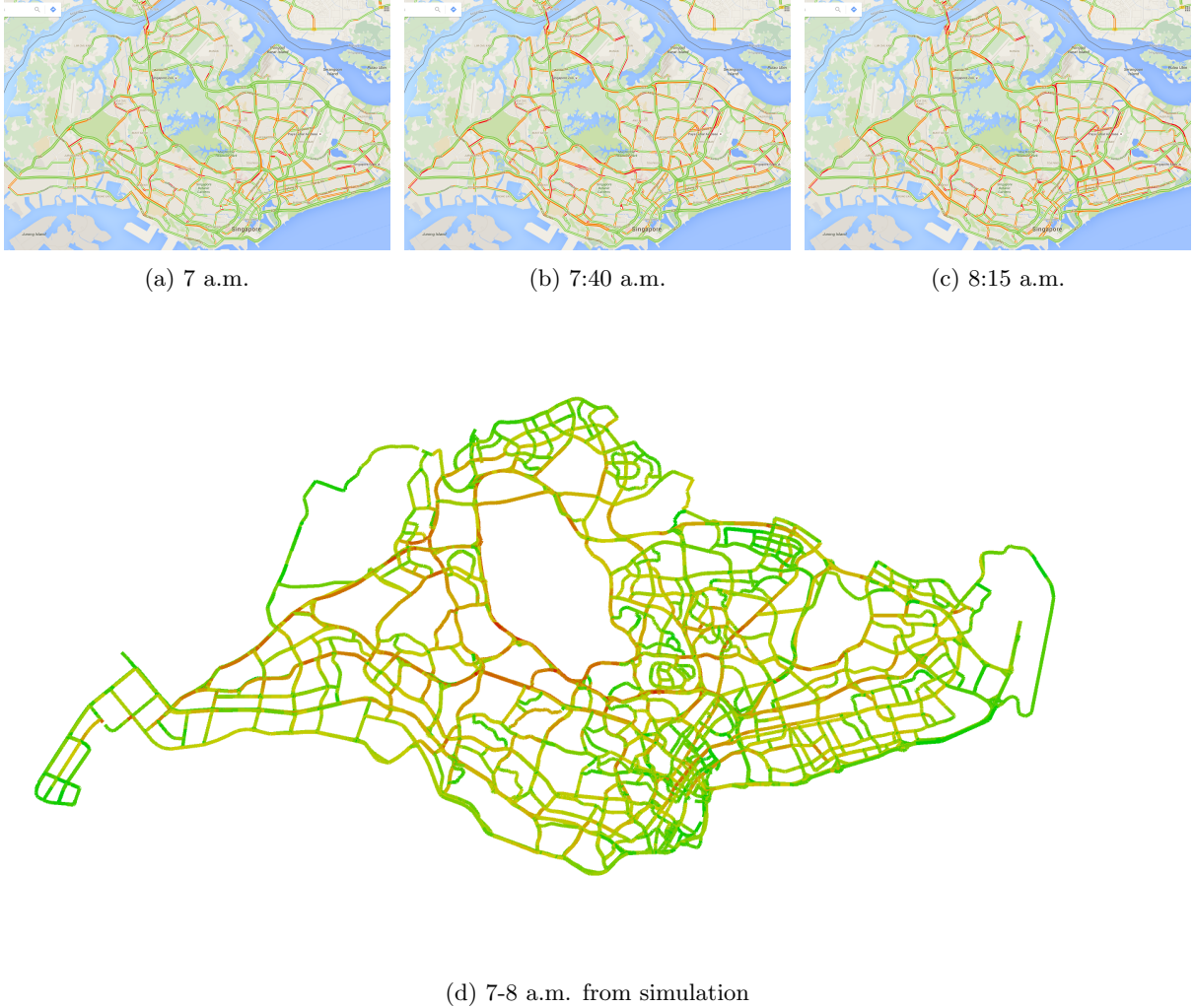
Figure 5: Comparison of congestion maps from our simulation 5d and Google Maps typical traffic service for 7 a.m. 5a, 7 : 40 a.m. 5b, and 8 : 15 a.m. 5c
