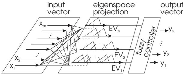
Figure 3: The structure of a fuzzy controller based on eigenspace projection.
