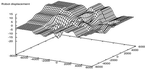
(b) Control surface with the first two eigenvalues as input and the robot displacement as output.
