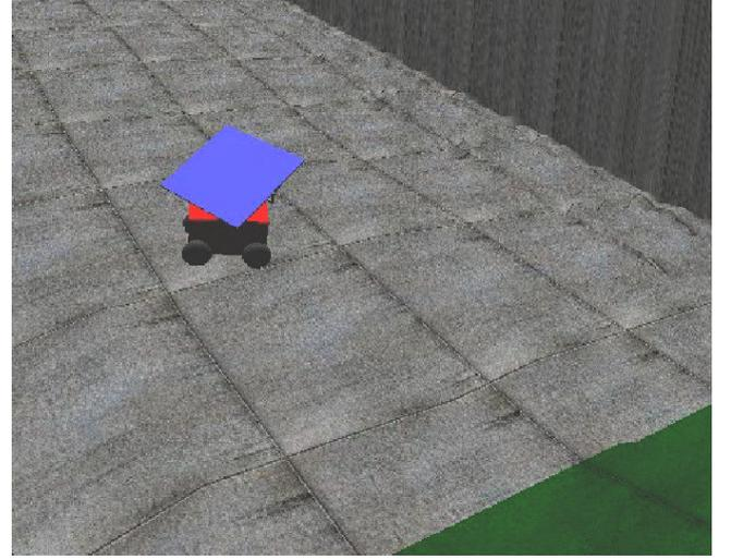
Fig. 7. The robot stopped here and is about to level the platform. The roll, pitch, yaw of the robot is (-23.2, -3.5, 65.5) and of the platform (-21.4, 33.3, 104.1). The platform and the robot are not aligned due to a previous rotation.
