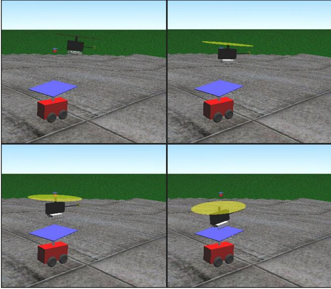
Fig. 4. Screenshots from a concept video. The modified ATRV-Jr is stopped on a slope with the platform leveled and a helicopter is on approach for landing.
