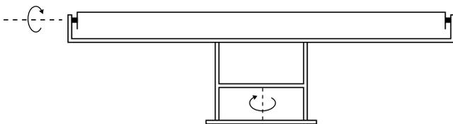
Fig. 1. Cross-section of a 2-axis gimballed platform design.
