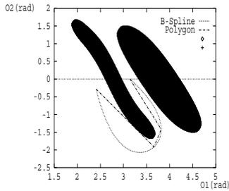
Fig. 5. Optimized trajectory through the subgoals in the c-space
