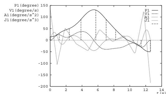
Fig. 4. Examples of optimizing a trajectory of a six joint PUMA robot - joint 1
