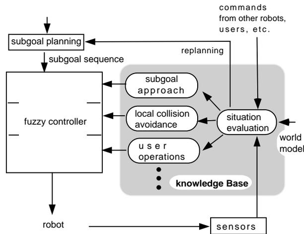
Fig. 1. Integration of subgoal planning and sensor-based plan execution.
