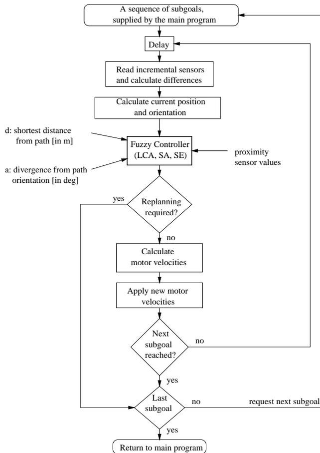
**Fig. 10.** Flow chart for integrating “subgoal planning” and “local collision avoidance”.
