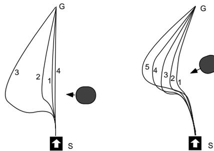
**Fig. 14.** Collision-avoidance with a dynamic obstacle.
