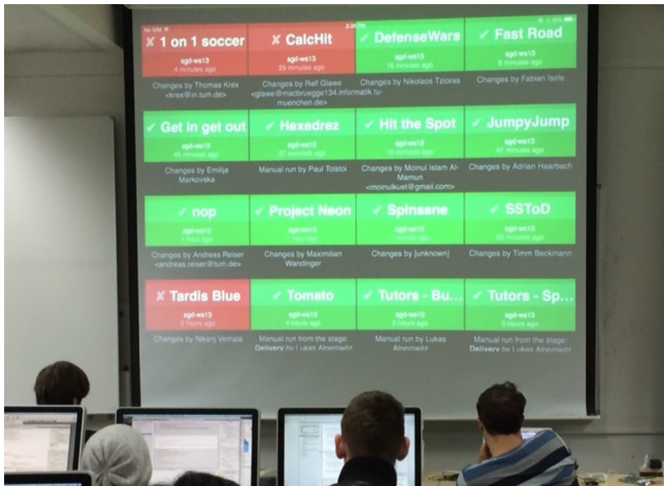
Figure 6.3: Wallboard showing whether the current version of the software is releasable or not
