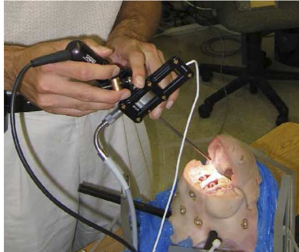
Fig. 7. Validation of the approach on a head of a pig cadaver with anatomical structures similar to the human sinuses. OptoTrak data is used as a ground truth to validate the motion estimation of our algorithm.
