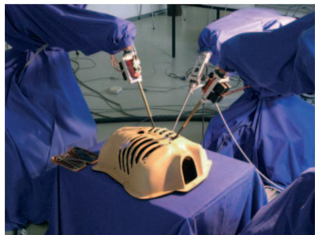
**Figure 4** Set-up with two surgical instruments and one camera port.
