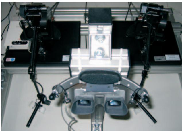
**Figure 3** PHANTOM<sup>®</sup> Devices for haptic feedback with head mounted display.
