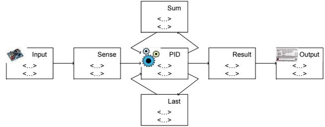
**Figure 2. Application Model: a PID Controller**
