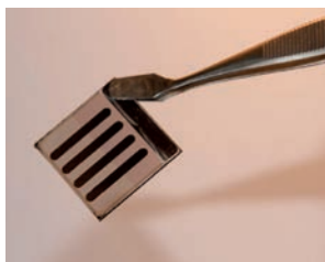
■ Example of polymer solar cell fabricated based on conjugated polymers and electron accepting small molecules.
