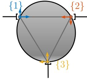
**Fig. 4.7:** Illustration of the kinematic grasp parameters for a planar manipulation task with  $N = 3$  manipulators
