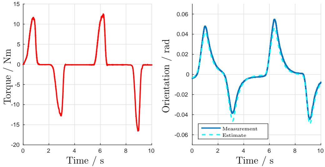
**Fig. 3.9:** Externally applied torque and resulting orientation about the z-axis
