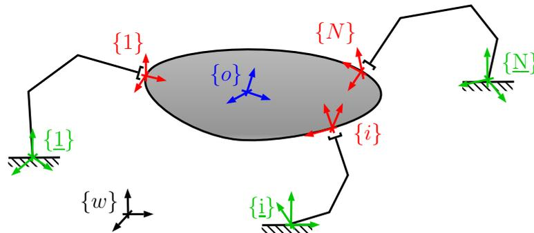
**Fig. 4.1:** Illustration of the local coordinate frames employed by the robotic manipulators for the cooperative manipulation task
