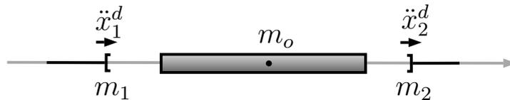
**Fig. 2.3:** Two cooperative manipulators handling a rigid object along one dimension
