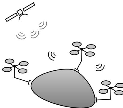
**Fig. 1.4:** Illustration of global and local localization systems for the coordination in a cooperative aerial manipulation task
