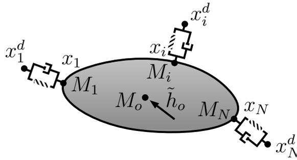
**Fig. 3.6:** Illustration of the apparent object dynamics as a parallel connection of mass-spring-damper elements
