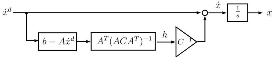
**Fig. 4.5:** Block scheme representation of the force/velocity cooperative manipulator model
