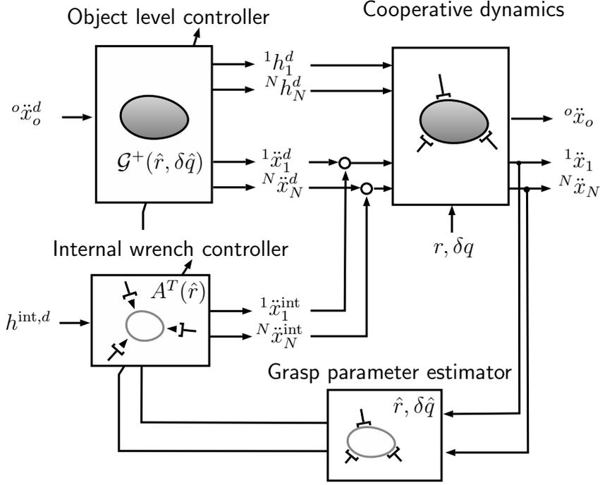
**Fig. 4.4:** Block scheme representation of the adaptive control law for robust force/motion tracking
