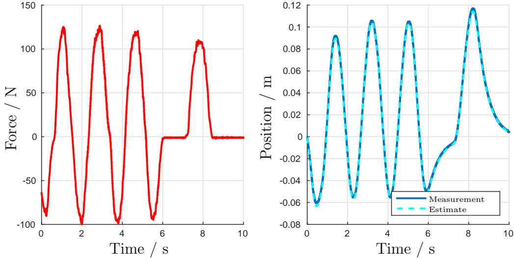
**Fig. 3.8:** Externally applied force and resulting position in x-direction
