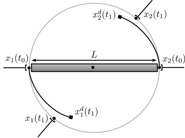
**Fig. 4.3:** Two planar manipulators with biased grasp parameter  $\hat{L} < L$  rotate a rigid bar counter-clockwise
