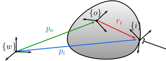
**Fig. 2.1:** Illustration of the coordinate systems employed for the cooperative manipulation task
