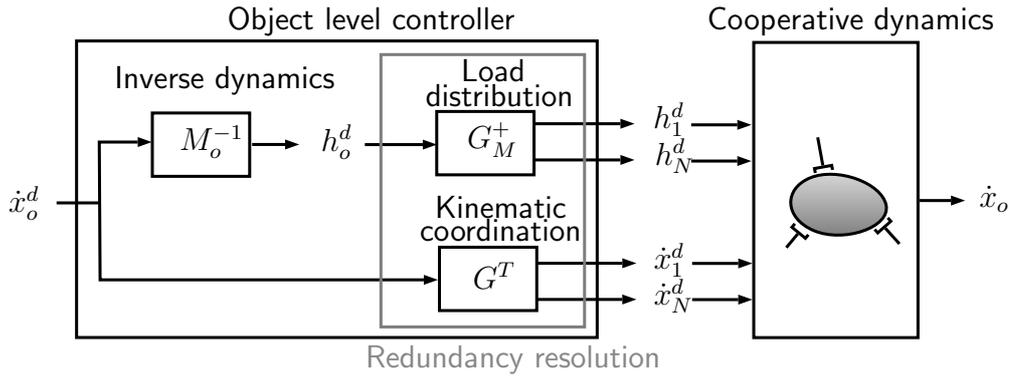
**Fig. 3.5:** Block scheme representation of controller and plant dynamics for cooperative force/motion tracking
