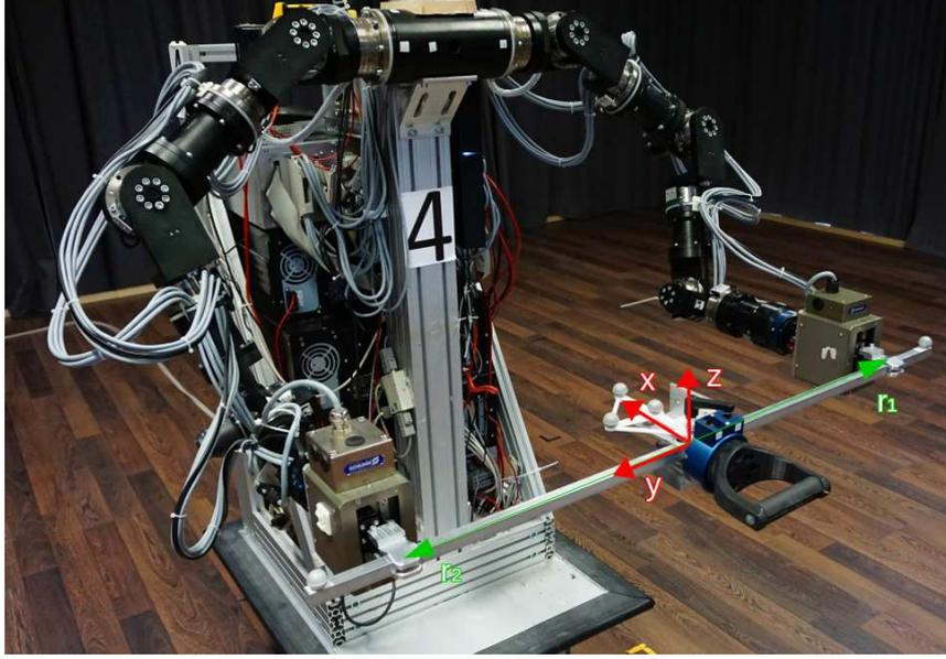
**Fig. 3.7:** Experimental setup with two robotic manipulators and force/torque sensor for measuring the externally applied wrench  $\tilde{h}_o$
