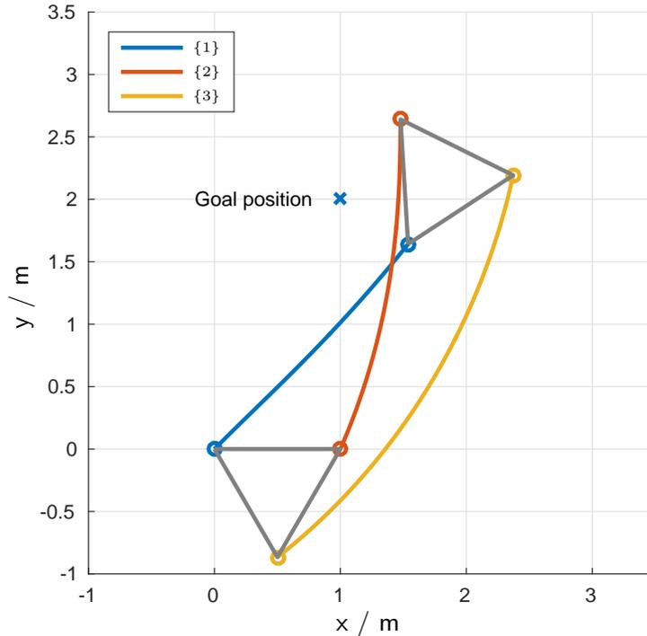
**Fig. 4.8:** Trajectory of the end effectors during the cooperative manipulation task
