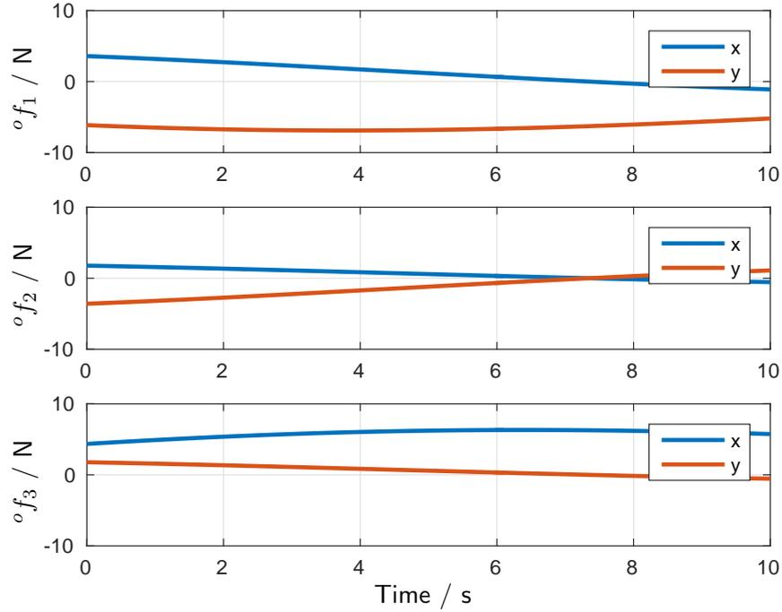
**Fig. 4.9:** End effector forces during the cooperative manipulation task without parameter adaptation
