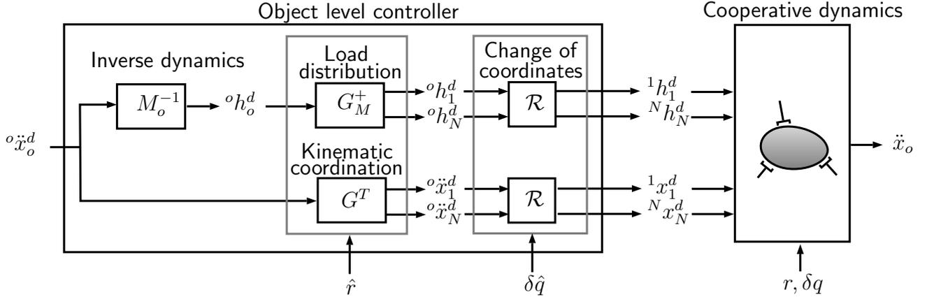
**Fig. 4.2:** Extended block scheme representation of the cooperative control system
