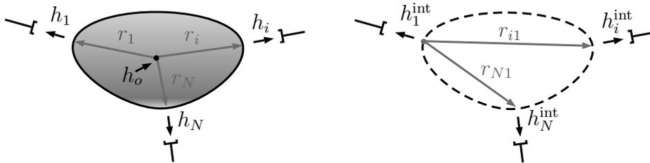
**Fig. 3.1:** Illustration of the constraining wrenches for the system of manipulators *plus* object and for the system of manipulators *without* object
