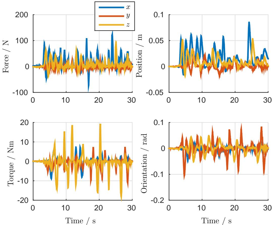
**Fig. 3.10:** Applied object wrench  $\tilde{h}_o$  and resulting object pose  $\delta x_o$  in  $SE(3)$
