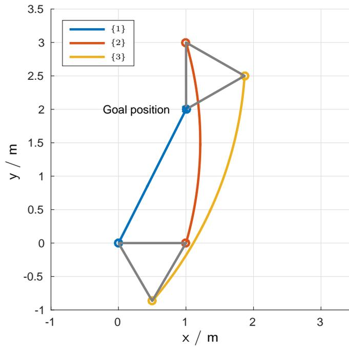
**Fig. 4.12:** Trajectory of the end effectors during the cooperative manipulation task with parameter adaptation
