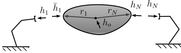
**Fig. 2.2:** Free-body diagram of the closed kinematic chain built by manipulators and object
