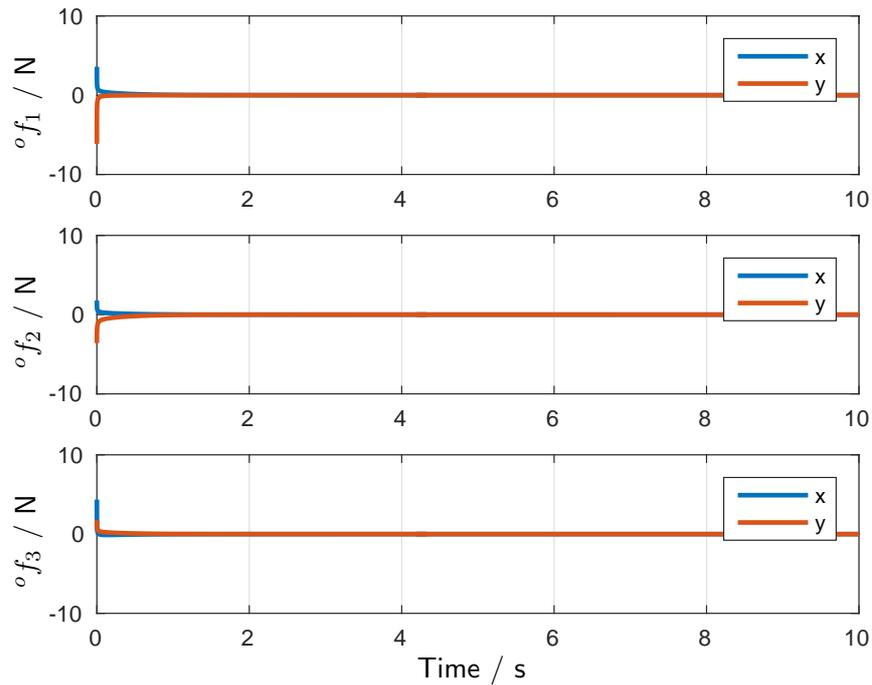
**Fig. 4.11:** End effector forces during the cooperative manipulation task with parameter adaptation
