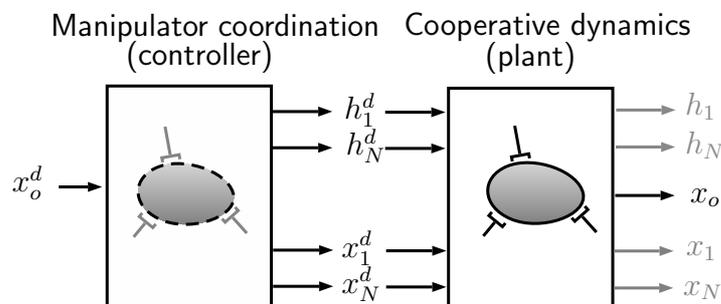
**Fig. 5.1:** Block scheme representation of the cooperative manipulator dynamics and the employed coordination strategy
