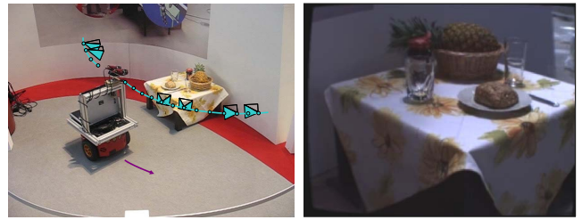
Fig. 5. (Left): Acquisition of a set of images with a stereo camera head mounted on a Pioneer 3-DX. (Right): A virtual image rendered from selected reference images. The virtual camera is placed at a position where there is no real camera.
