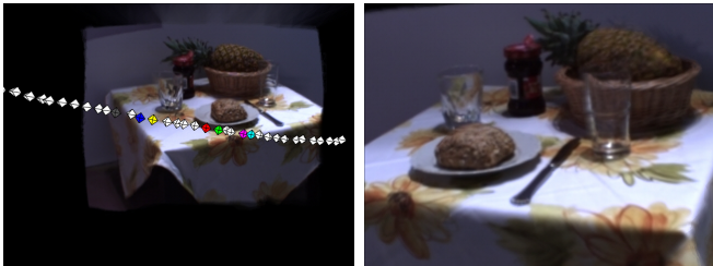
Fig. 8. (Left): A virtual image which shows apart from the scene some of the reference cameras which are depicted by a part of their viewing frusta. The colored reference cameras are chosen by the view selection algorithm and contribute to rendering this virtual image. (Right): A close-up virtual view onto the objects of interest.
