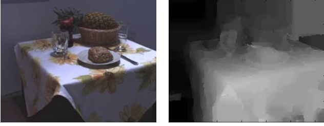
Fig. 2. A reference image (left) together with its computed depth map (right). High intensity values represent scene points which are near to the camera, low intensities correspond to far scene points.
