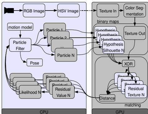
Figure 4: Scheme of the proposed tracking system, illustrating the subdivision of tasks between the CPU and the GPU.
