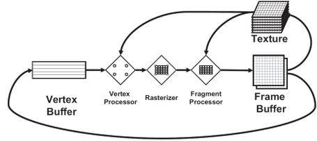
Figure 3: Graphics hardware pipeline. Image taken from [15]
