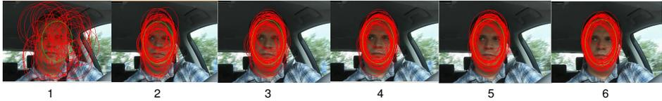
Figure 6: Condensation of the particle set after re-initialization.
