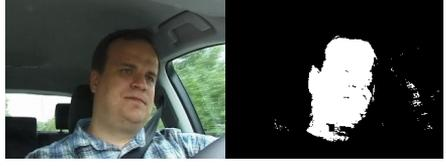
Figure 1: An input video frame and the corresponding segmented image using GMM.
