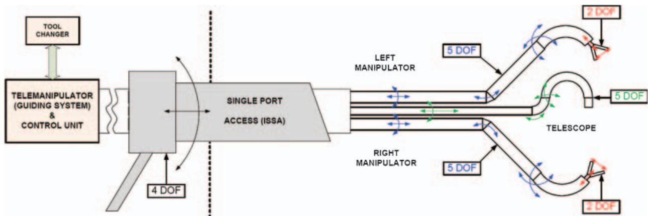
Figure 1. Schematic drawing of the “Highly Versatile Single Port System”
