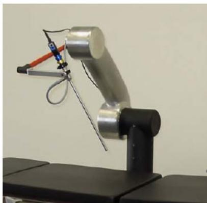
Figure 1 - SOLOASSIST is a mechatronic system providing camera guidance during minimally invasive surgical intervention. This system allows a 360° circle range in conjunction with an 80° inclination of the endoscope.
