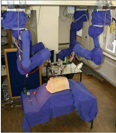
Fig. 2: Experimental robotic platform with integrated haptic feedback (new system)
