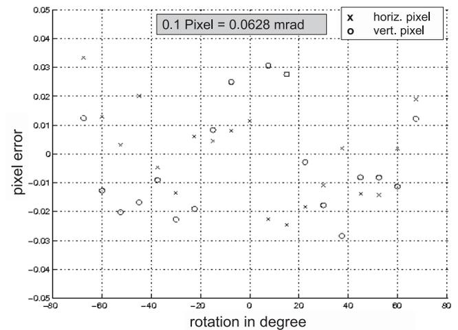
Figure 12: Remaining pixel error of the simulated target with respect to the rotation of the target.
