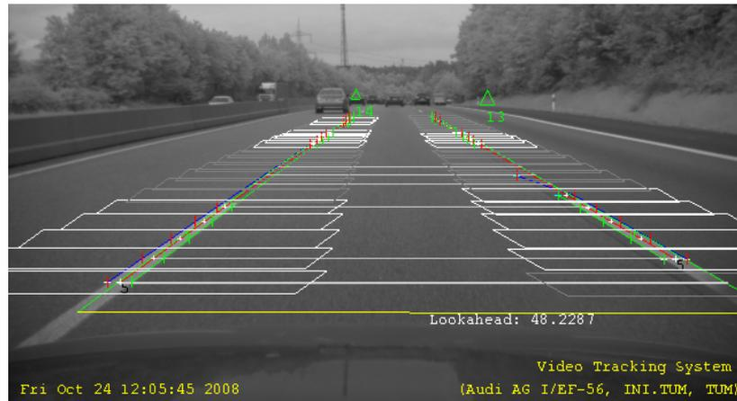
**Figure 3: Lane tracking on a real image**
