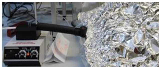
Figure 7 Injection of a mixture of water-target compounds 4-OPA, IPOH, 4-AMCH in TBs with the scope to generate gaseous atmosphere. On the left side: the heater and on the right side: the TBs protected from light with aluminium foil
