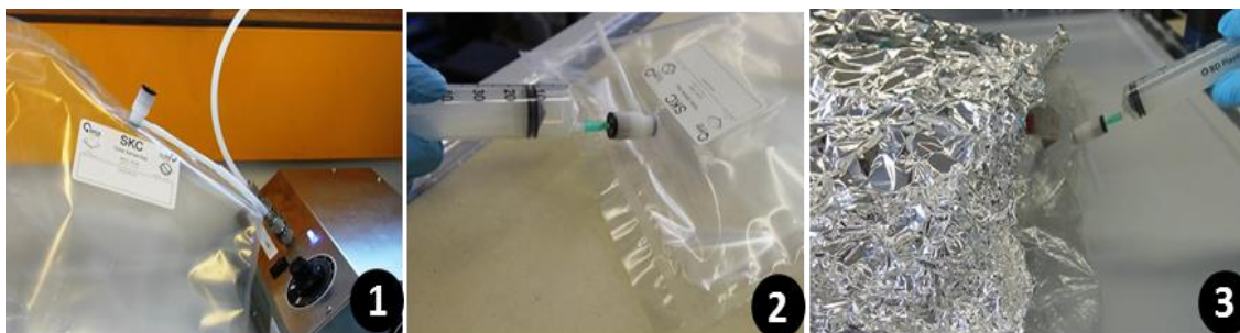
Figure 8 Main steps involved in the generation of gas mixture atmospheres in TBs: 1. Ozone generator; 2. Sampling of ozone with the PP syringe; 3. Injection of ozone in the TBs already containing the mixture of 4-OPA+IPOH+4-AMCH
