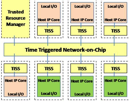
Fig. 2. Hardware Architecture
