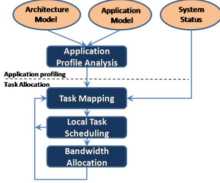
Fig. 3. Task Allocation Flow
