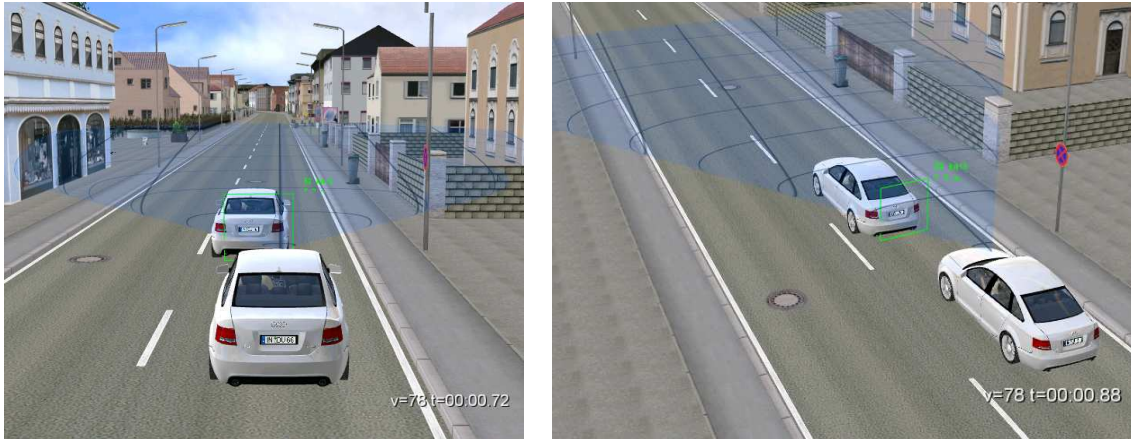
Figure 6: Sensor cone for the virtual pre-crash-sensor
