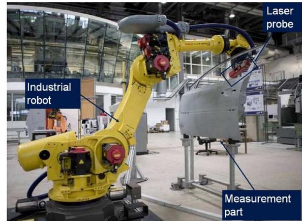
Fig. 15. Robot-guided optical scanning devices.
