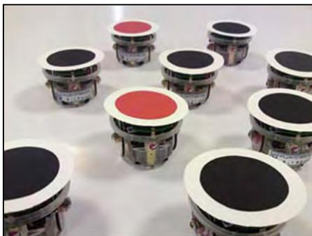
Figure 1. Experimental setup, 9 E-Pucks were used in this work, Informed agents were capped in red and naïve agents were capped in black labels.
