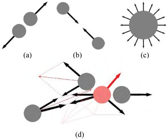
Figure 3. Potential field vectors for flock formation, (a) Separation vector, (b) Cohesion vector, (c) A random vector representing movement of the robots in a random direction, (d) Calculation of resultant vector, shown by light red vectors. The heavy red vector depicts the direction of target used by informed robots (specified by a red circle).
