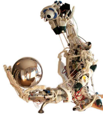
Fig. 1. ECCE-I PROTOTYPE. Prototype of the anthropomorphic [12] robot ECCE-I developed within the EU-funded project ECCEROBOT [5, 13]. The skeleton is hand-crafted using polymorph—a caprolactone polymer—which can easily be molded. The human muscles are imitated by elastic, tendon-driven actuators comprising a DC motor and a gearbox in series with a kite line and shock cord that function as the muscle fibers and tendon, respectively.
