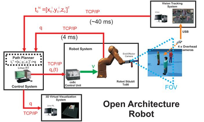
Fig. 5. Human Tracking System Block Diagram
