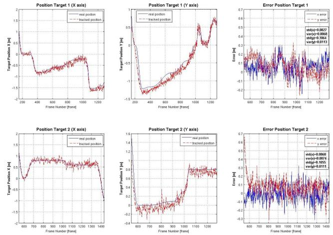
Fig. 9. Tracking Results with respect to the ground truth using the animated scene. It shows the tracking results for the two target in  $X$  and  $Y$  along with the standard deviation and variance of the result.
