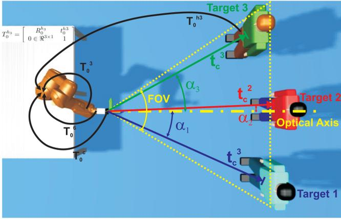
Fig. 6. Camera's Field of View and the Eye in Hand camera.
