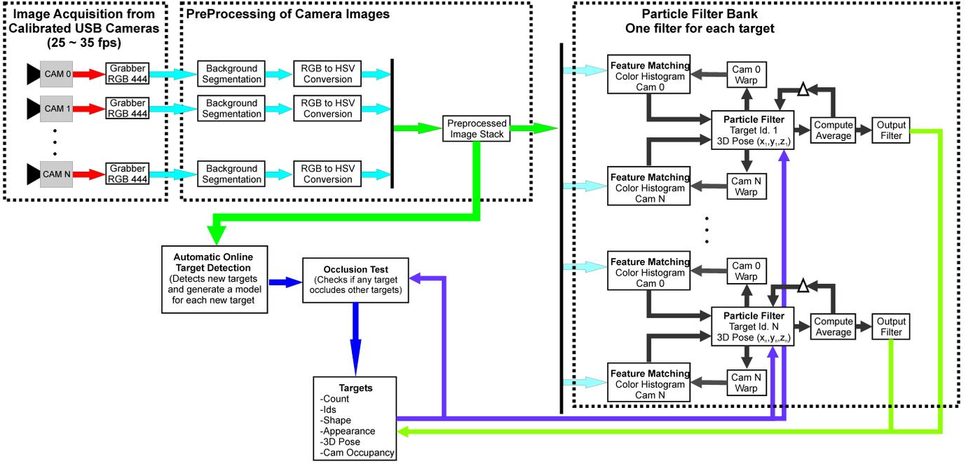
Fig. 2. The figure illustrates the block diagram of the tracking system. It consists of the image acquisition module, target detection module, occlusion test module and the particle filter bank.
