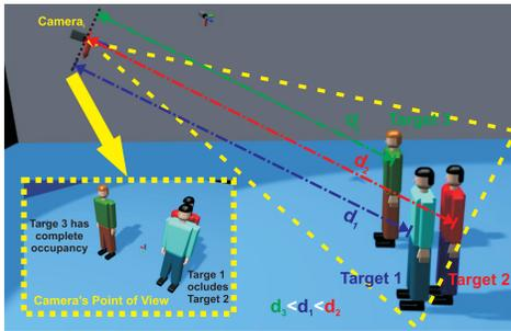
Fig. 3. The figure illustrates the occlusion test system. The left part of the figure shows a scene in a camera view with 3 targets, where target 1 occludes target 2. The right part of the figure shows how the occlusion is detected by rendering the targets with respect to their distance from the camera. The target closest to the camera is rendered first.
