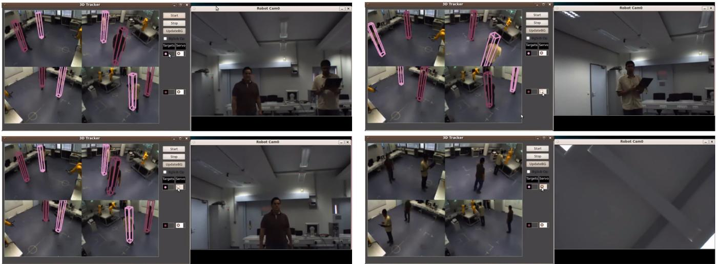
Fig. 10. The figure illustrates the test results. The 4 clustered images represent the tracking system results along with an additional robot mounted camera output. **Top Left:** Two targets are tracked and served by the robot. **Top Right:** Only target 1 is enabled to be served by the robot. **Bottom Left:** Only target 2 is enabled to be served by the robot. **Bottom Right:** Target 1 gets closer than the safety limit of the robot and robot goes to park position and all systems are shutdown.
