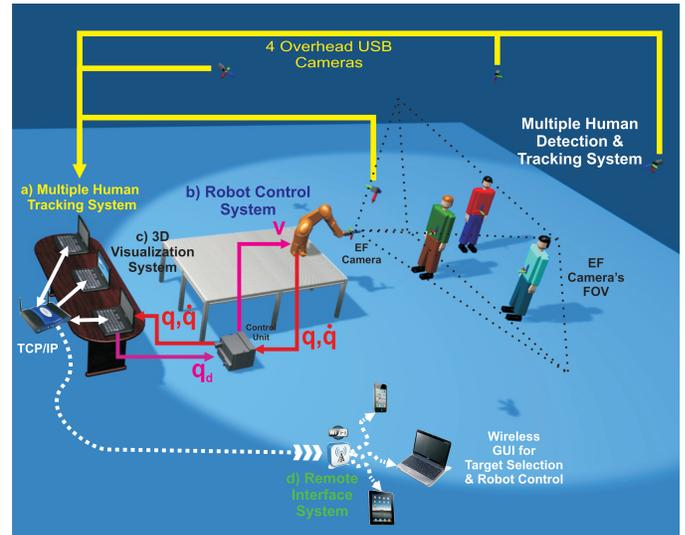
Fig. 1. Complete Robotic Setup. The figure shows the different systems involved in the robotic setup. a) the Multiple Human Tracking System: 4 USB cameras connected to a GNU/Linux OS PC, b) Robot Control System: An industrial robot StäubliTX90 and a CS8C control unit are connected to a GNU/Linux RT OS PC, c)3D Visualization System: OpenGL-based virtual world visualization running on a GNU/Linux PC and d) Remote Interface System: it allows the user to select the targets and control the robot.
