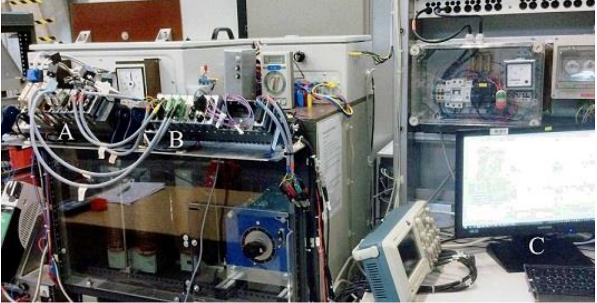
Fig. 2.11: FPGA HiL platform of a back-to-back power converter PMSG wind turbine system. A : FPGA platform (NI-cRIO-9082), for implementing the ECU; B : FPGA platform (NI-9159), for implementing the back-to-back converter PMSG wind turbine emulator; C : User interface, programmed using Labview running in a PC.
