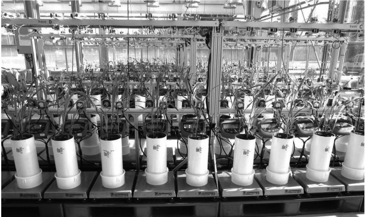
Figure 3 Greenhouse trial conducted in the Phenodyn facility in Montpellier. Four maize plants were initially grown per pot. The experimental design integrates automatized weighing of pots.
