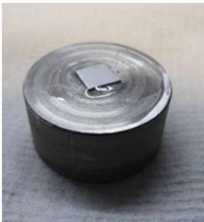
Figure 5.8: Fuel sample glued in an Al block with hardened crystal bond.
