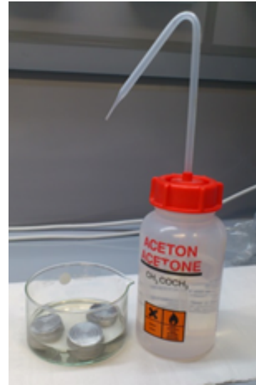
Figure 5.11: Removing the fuel sample from the Al block with acetone.
