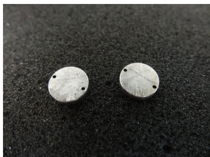
Figure 4.7: Platinum lids with two holes to flood the crucibles with purging gas [Rei13].
