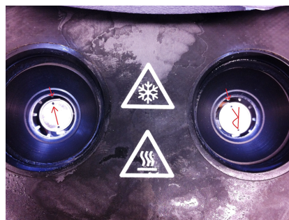
Figure 4.8: The red marks show how the lids are engraved for better alignment [Rei13].
