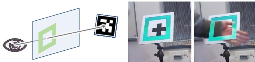
**Figure 1.8:** An example of an OST AR application with our OST-HMD. The system tracks the position of a physical square marker in the scene, and it renders a virtual green frame aligned on the marker from the user-perspective view. We used a see-through head-mounted display for the rendering.
