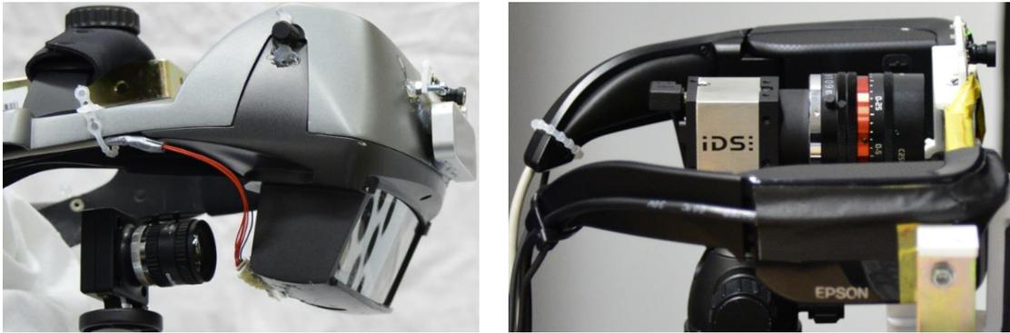
**Figure 10.2:** Hardware setup. (Left) nVisor ST60. (Right) Moverio BT-100. The camera on the left image is displaced for the photography; it was set closer to the screen during actual data collections.
