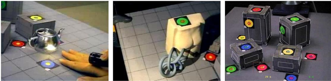
**Figure 1.5:** A vision-based AR application from a pioneering work by State et al. presented in 1996 [Sta+96]. The system integrates virtual models in the real world. Its tracking is based on prediction of concentric circular dots and a magnetic tracker.
